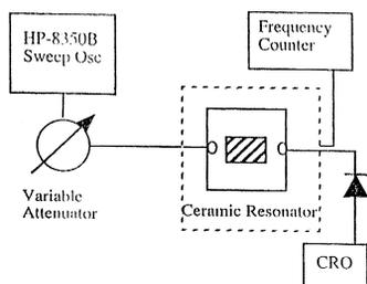
Fig. 2. Schematic diagram of the experimental set-up used for the WGM measurements.
