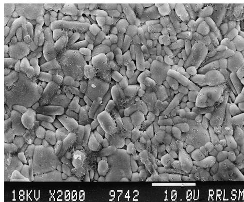
Fig. 3. SEM picture recorded from  $\text{BaCe}_2\text{Ti}_5\text{O}_{15}$  ceramic.
