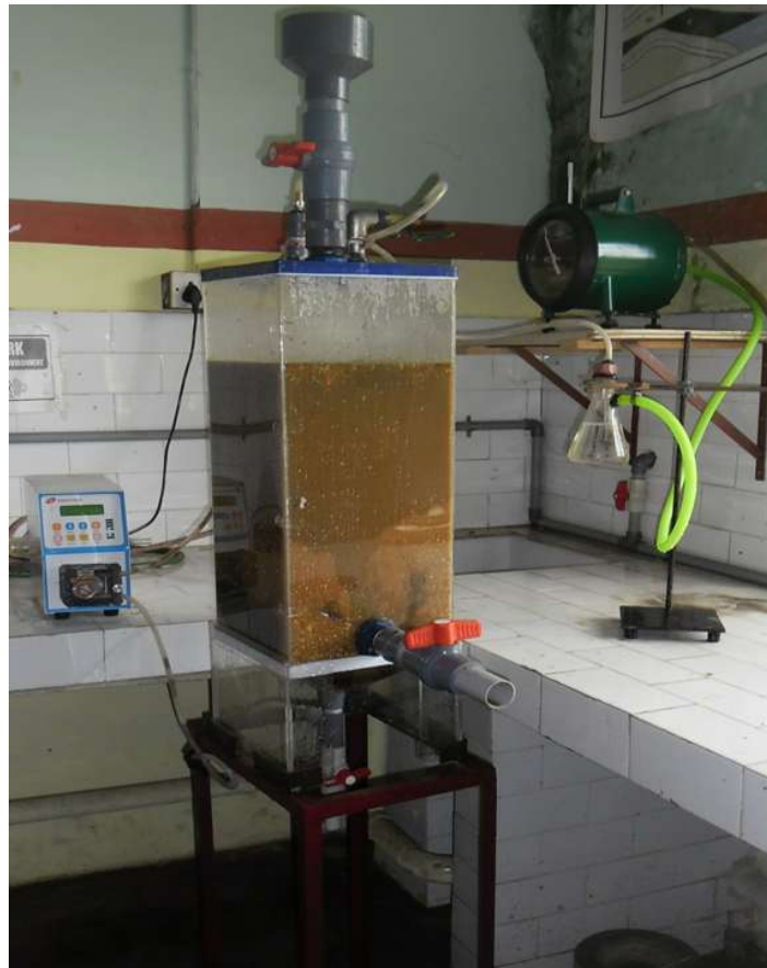
Figure 3.6 Experimental setup of semi-dry anaerobic digester for continuous study
