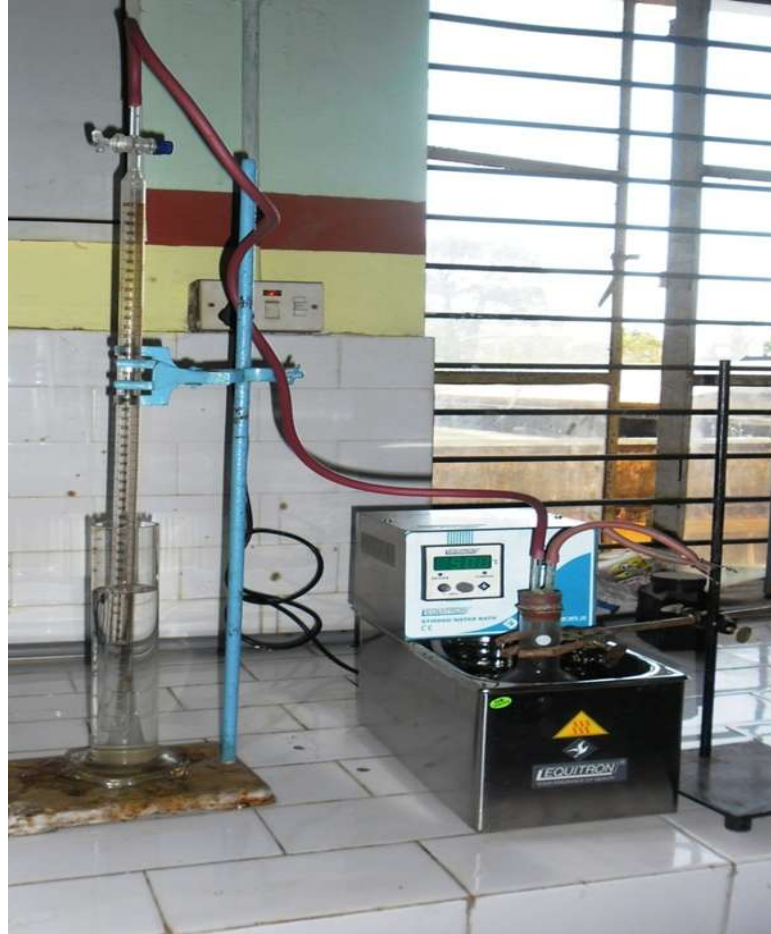
Figure 3.4 Experimental setup of batch study at thermophilic temperature
