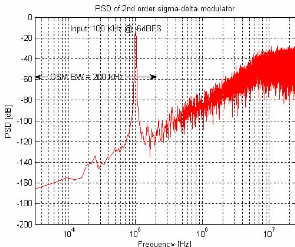
(a) Modulator output spectrum in GSM mode
