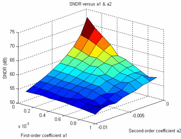
Figure 4. 3D Simulation for non-linear dc gain
