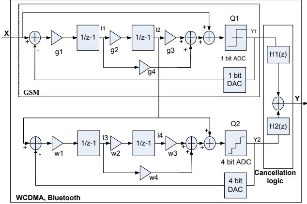
**Figure 2. Block diagram of a triple-mode sigma-delta modulator**
