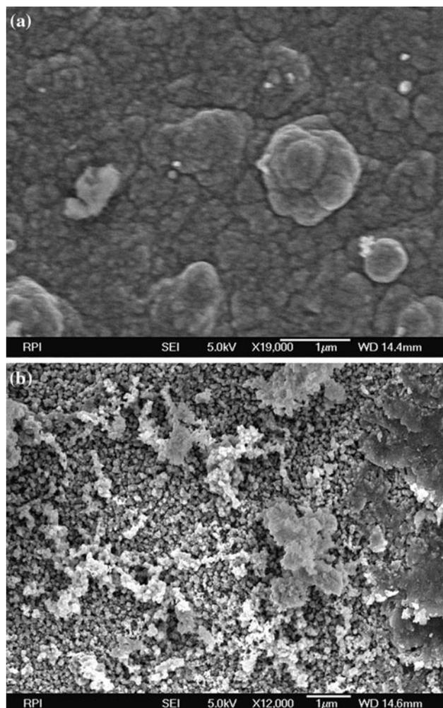
**Fig. 8** **a** SEM images of SAC-12 and **b** WAC-8 nanocomposites
