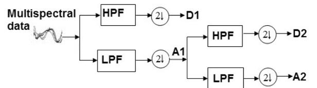
Fig. 2. Wavelet Analysis of multispectral data
