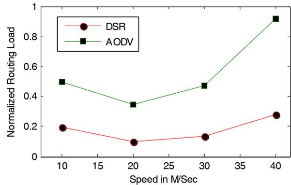
Fig. 6. Normalized routing load against Speed variations for freeway model
