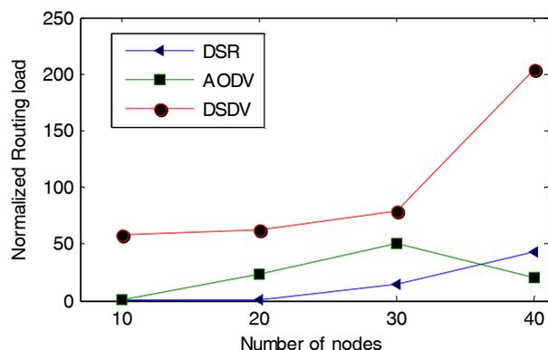
Fig. 7. Normalized routing load against number of mobile nodes for freeway model
