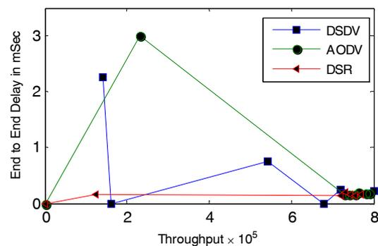
Fig. 2. End-to-End delay variations against throughput in RPGM mobility model
