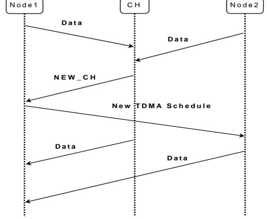
Figure 2. Network operation of static-EACM
