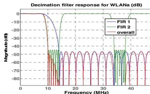
Figure 6. Decimation filter response for WLANa
