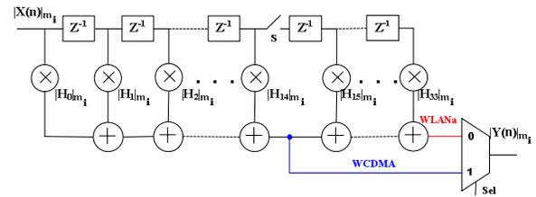
Figure 4.  $i^{\text{th}}$  filter channel of stage 1
