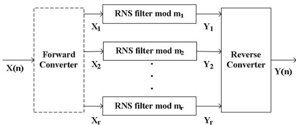
Figure 1. RNS based FIR filter
