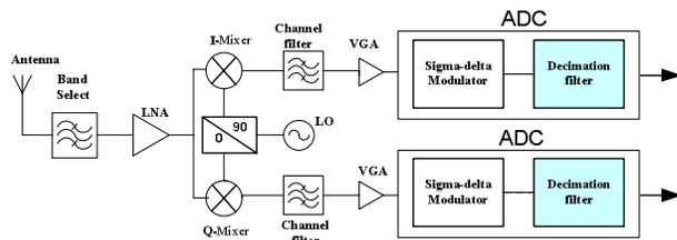
Figure 2. Direct conversion homodyne receiver architecture
