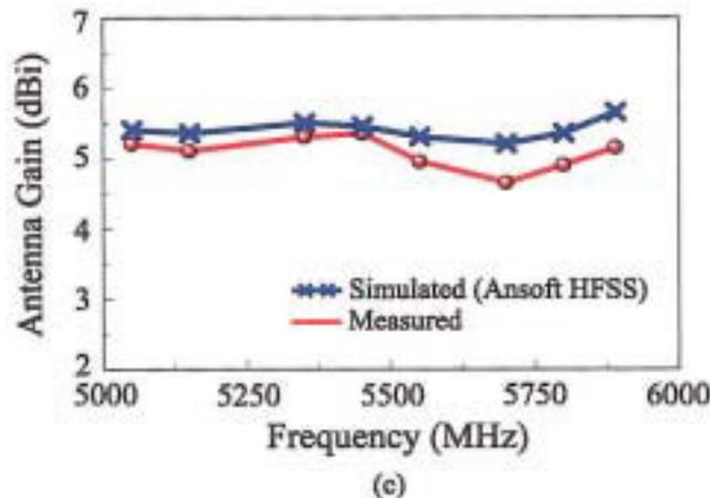
**Figure 8** Measured and simulated antenna gain vs. frequency for (a) the first resonant mode, (b) the second resonant mode, and (c) the third resonant mode. [Color figure can be viewed in the online issue, which is available at [www.interscience.wiley.com](http://www.interscience.wiley.com)]
