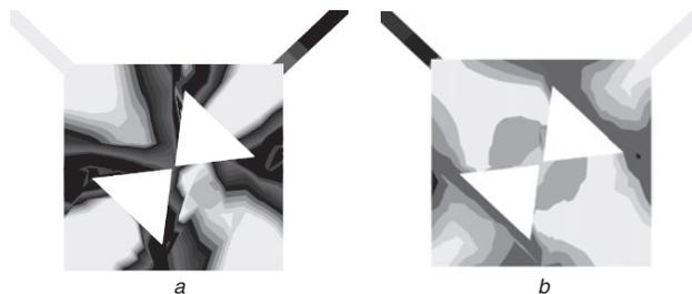
Fig. 2 Current path on patch
