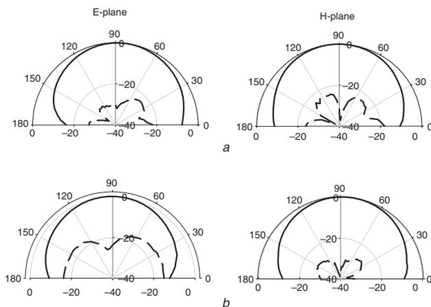
**Fig. 5** E-plane and H-plane radiation characteristics of proposed antenna
