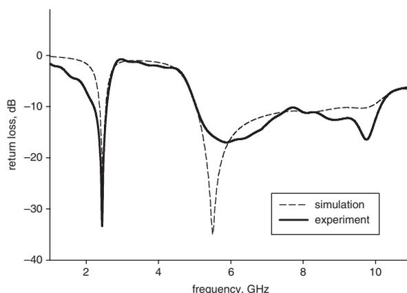
Fig. 2 Simulated and measured return loss characteristics of antenna structure
