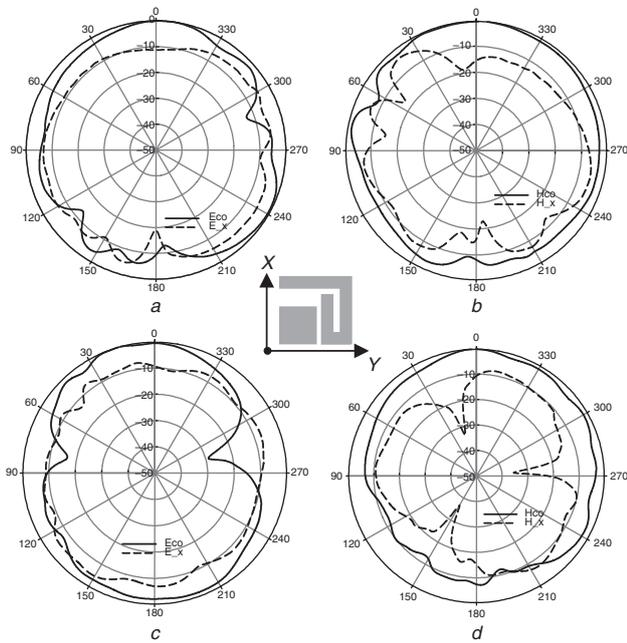
**Fig. 4** Measured radiation patterns
