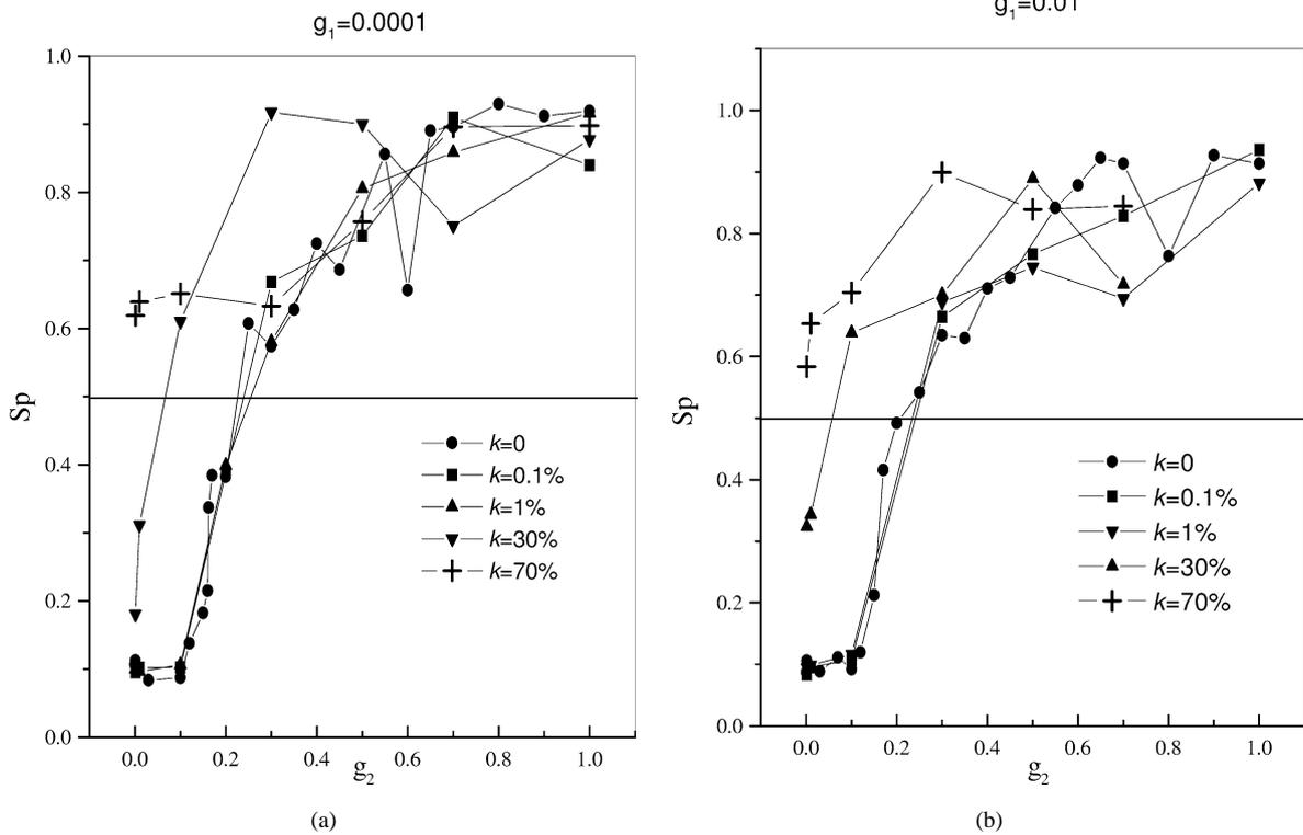
Fig. 7. The dependence of phase synchronization on the coupling factor  $g_2$  in the presence of various noise levels,  $k$ , in the case of uniformly distributed noise with finite mean for the mutually coupled systems at two feed forward coupling values. (a)  $g_1 = 0.0001$  and (b)  $g_1 = 0.01$ .
