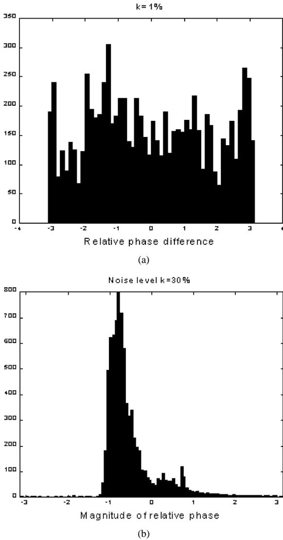
Fig. 3. The distribution of the relative phase difference in the weakly coupled system with  $g_1 = 0.0001$  and  $g_2 = 0.001$ . The additive noise of finite mean is added to a level of (a) 1% and (b) 30%.
