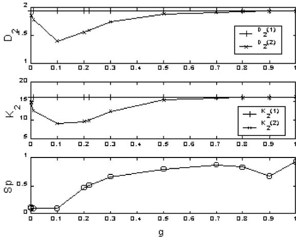
Fig. 1. The variations in  $D_2$ ,  $K_2$  and  $Sp$  with the coupling factor  $g$  for a uni-directionally coupled Rossler system. 1 refers to the drive system and 2 to the response.
