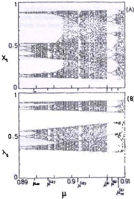
Fig. 1. Bifurcation structure of MLM for the parameter range  $0.89 < \mu < 0.91$  projected (A) onto the  $(X_t, \mu)$  plane and (B) onto the  $(\lambda_t, \mu)$  plane which is just the bifurcation structure of the logistic map for the specified range of the parameter.
