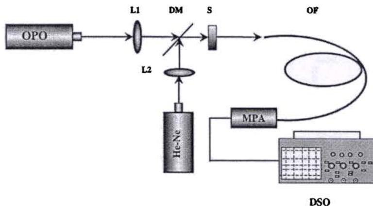
Fig. 1. Schematic diagram of the experimental set up.  $L_1$ ,  $L_2$  - Lens; DM - Dichroic Mirror; S - Sample; OF - Optic Fibre; MPA - Monochromator - PMT assembly; DSO - Digital Storage Oscilloscope.
