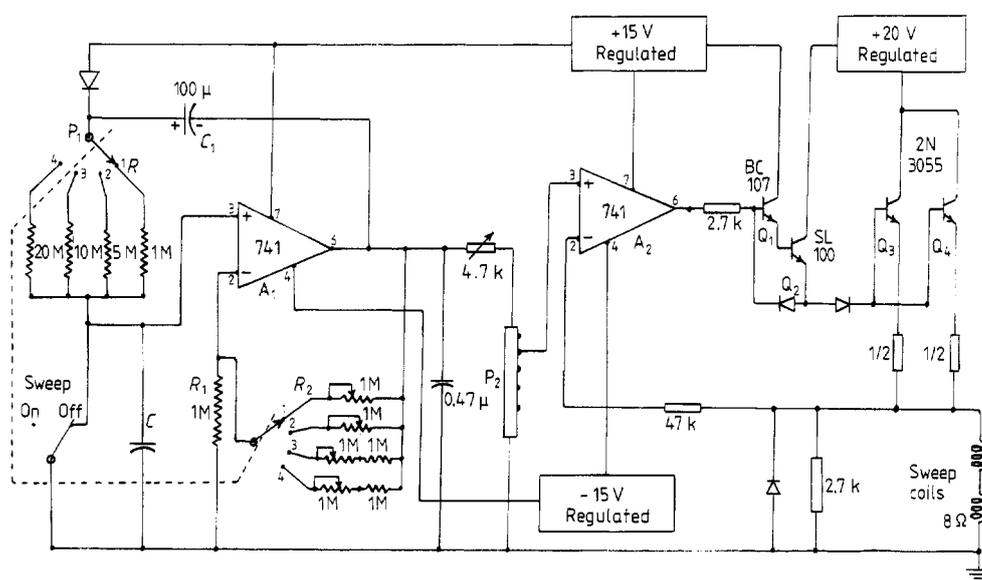
Figure 1. Schematic circuit of the field sweep generator.
