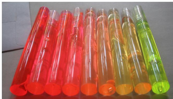
Fig. 1. A photograph of the fabricated preforms.
