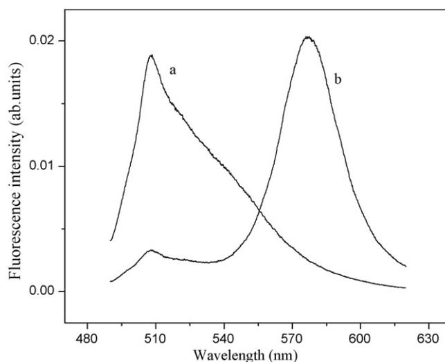
Fig. 5. Variation of fluorescence intensities: (a) fluorescein alone and (b) fluorescein-rhodamine B system.
