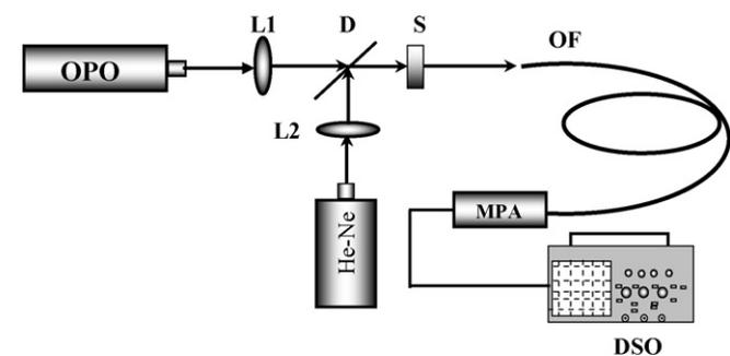
Fig. 1. Schematic diagram of the experimental set up. L<sub>1</sub>, L<sub>2</sub>, lens; DM, dichroic mirror; S, sample; OF, optic fibre, MPA, monochromator-PMT assembly; DSO, digital storage oscilloscope.
