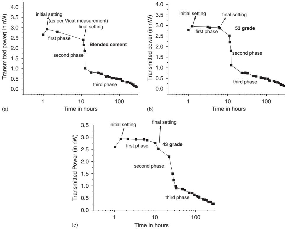
Fig. 4. A typical graph showing time vs. intensity of a cement sample.
