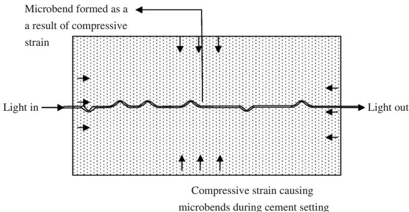
Fig. 1. Stress-induced microbends in an optical fiber.
