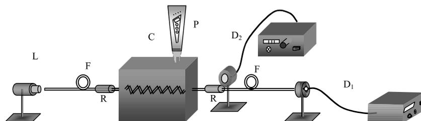
Fig. 1. Schematic diagram of the experimental set-up L: diode laser (633 nm), C: cell containing pH solution, P: pH electrode, F: optical fiber, R: index matching liquid  $D_1$ : detector 1 (Metrologic 45–545),  $D_2$ : detector 2 (Newport 1815-C).
