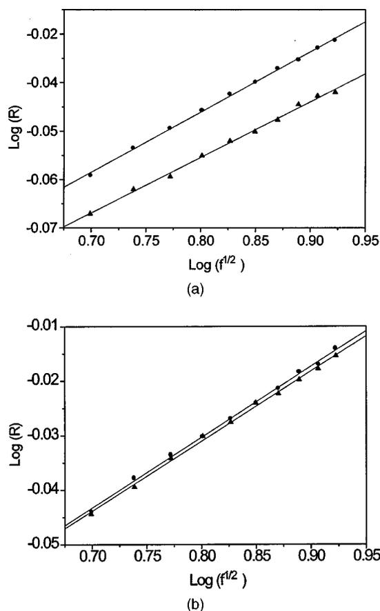
**Fig. 5** Logarithmic plot connecting the square root of frequency  $f$  and the amplitude ratio  $R$  for: (a) BL001 and BL002 with the reference sample (Cu foil), the solid triangle is for BL001 and the solid circle is for BL002, and (b) for BL032 and BL035 with the reference sample (Cu foil), the solid triangle is for BL032 and the solid circle is for BL035.
