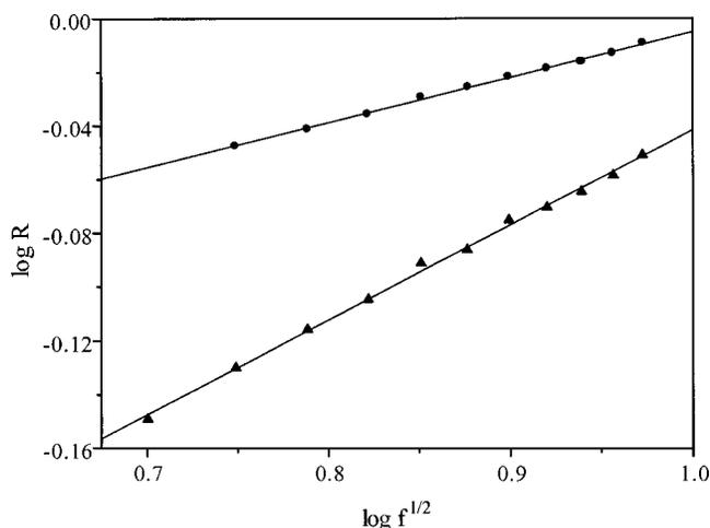
**Fig. 4** Logarithmic plot connecting the square root of frequency  $f$  and the amplitude ratio  $R$  for water and glycerol with the reference sample (Cu foil). The solid circle is for glycerol and the solid triangle is for water.
