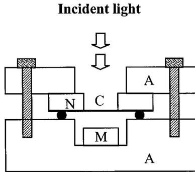
Fig. 1 Cross-sectional view of the OPC: A=acrylic frame; M=microphone; N=nylon ring; and C=copper foil.
