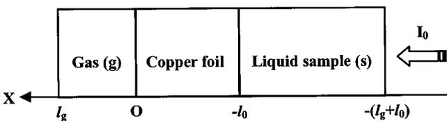
Fig. 2 Schematic diagram of the geometry of the OPC for which the calculations were made. The periodic heat is generated at  $x = -l_0$ . For an empty sample holder, the liquid sample  $s$  is replaced with the gas  $g$ .
