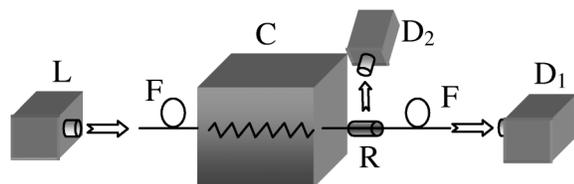
Fig. 2. Schematic diagram of the experimental setup: L, diode laser (670 nm); C, cell containing MB in water; Fs, optical fibers; R, index-matching liquid; D<sub>1</sub>, detector 1 (Metrologic 45-545); D<sub>2</sub>, detector 2 (Newport 1815-C).
