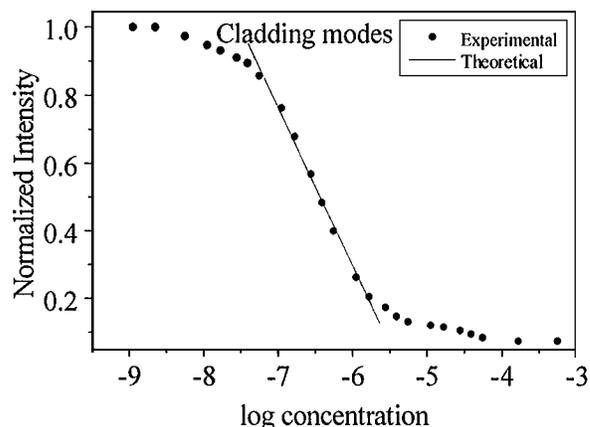
Fig. 4. Cladding-mode intensity variation with dye concentration.
