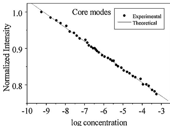
Fig. 3. Core-mode intensity variation with dye concentration.
