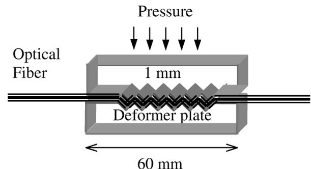
Fig. 1. Schematic diagram of the setup used to deform the optical fiber.
