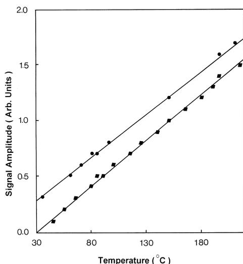
Fig. 2. The plot of the signal vs. temperature for the heating element. (● Heating; ◆ Cooling).
