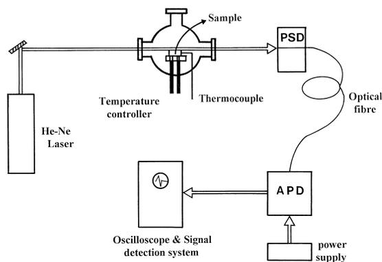
Fig. 1. Schematic diagram of the experimental set-up using the single beam method.
