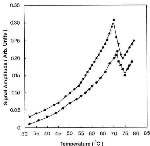
Fig. 3. The plot of the signal vs. temperature for liquid crystal  $E_8$ .  $T_{NI} = 70.0^\circ\text{C}$  (● Heating; ◆ Cooling).
