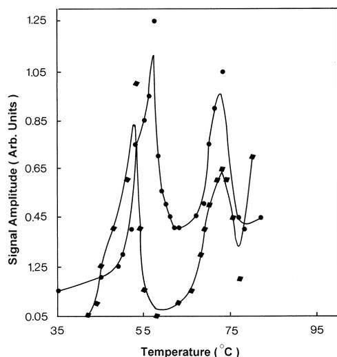
Fig. 4. The plot of the signal vs. temperature for liquid crystal  $M_{21}$ .  $T_M = 55.0^\circ\text{C}$ ,  $T_{NI} = 73.5^\circ\text{C}$  (● Heating; ◆ Cooling).
