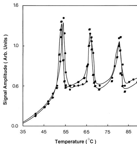
Fig. 5. The plot of the signal vs. temperature for liquid crystal  $M_{24}$ .  $T_M = 54.0^\circ\text{C}$ ,  $T_{AN} = 67.5^\circ\text{C}$ ,  $T_{NI} = 80.5^\circ\text{C}$  (● Heating; ◆ Cooling).
