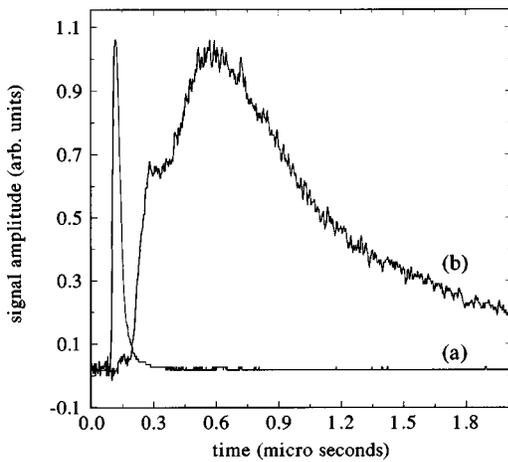
FIG. 2. Temporal profiles of (a) the emission from  $N_2^+$  at 427.8 nm and (b) that of silver atomic emission at 546.5 nm.
