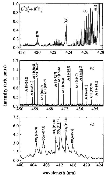
FIG. 4. Time resolved spectra with different ambient atmospheres with a gate delay 0 ns and width 40 ns. (a) High resolution spectrum of the emission  $\Delta v = -1$  band from  $N_2^+$ . Spectrum shows clearly resolved rotational lines with intensity alternations. (b) The spectrum with argon ambient where the spectrum is dominated by the emission from singly ionized argon. (c) The spectrum of carbon dioxide obtained under the same pressure conditions as that for nitrogen ambient.
