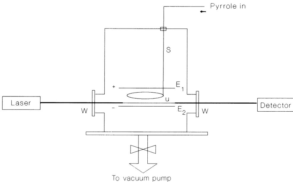
Fig. 1. Schematic of the experimental set-up. W, window; E, electrode; s, sprayer; u, uncladded region of the fibre.
