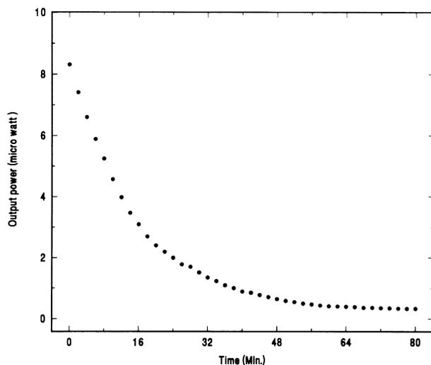
Fig. 2. Typical plot of output power variation with time.
