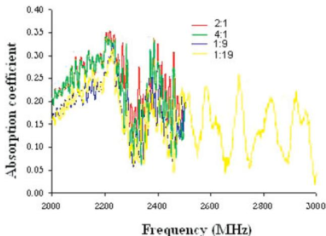
**Figure 5** Variation of absorption coefficient with frequency of HAP-chitosan composite. [Color figure can be viewed in the online issue, which is available at [www.interscience.wiley.com](http://www.interscience.wiley.com)]
