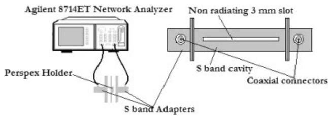
Figure 1 Experimental setup
