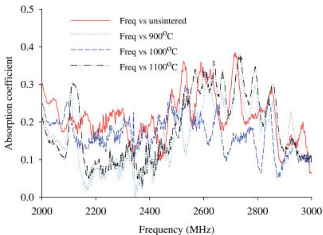
**Figure 4** Variation of absorption coefficient with frequency of HAP powder at different sintering temperatures. [Color figure can be viewed in the online issue, which is available at [www.interscience.wiley.com](http://www.interscience.wiley.com)]
