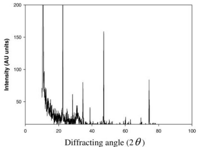
**Figure 2** XRD of unsintered HAP
