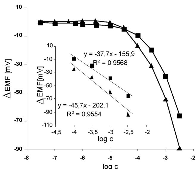
Fig. 2. Potentiometric response toward paracetamol of Mn(III)-porphyrin ISE (■) and Mn(III)-porphyrin CPE (▲). The measurements were performed in the presence of  $1.0 \times 10^{-2}$  M phosphate buffer, pH 5.5 (■,  $n = 8$ ;  $0.24 < SD < 9.35$ ), (▲,  $n = 6$ ;  $0.25 < SD < 11.92$ ).
