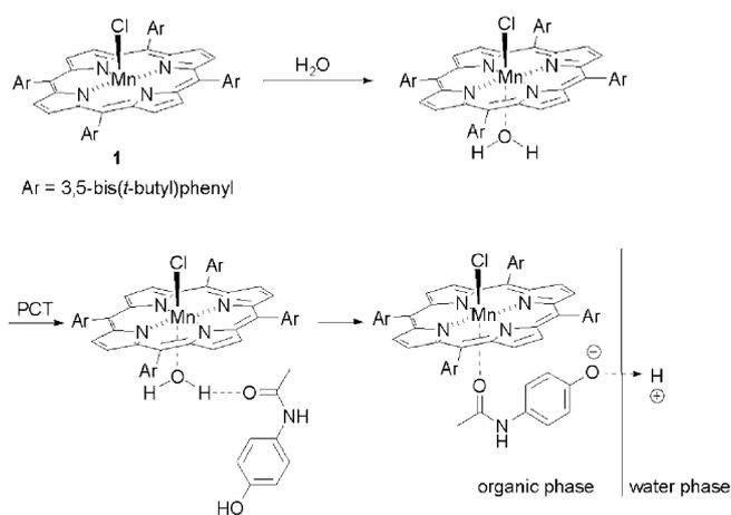
Scheme 1. The illustration of the mechanism of potentiometric signal generation by potentiometric sensors incorporating Mn(III)-porphyrin in the presence of undissociated paracetamol.
