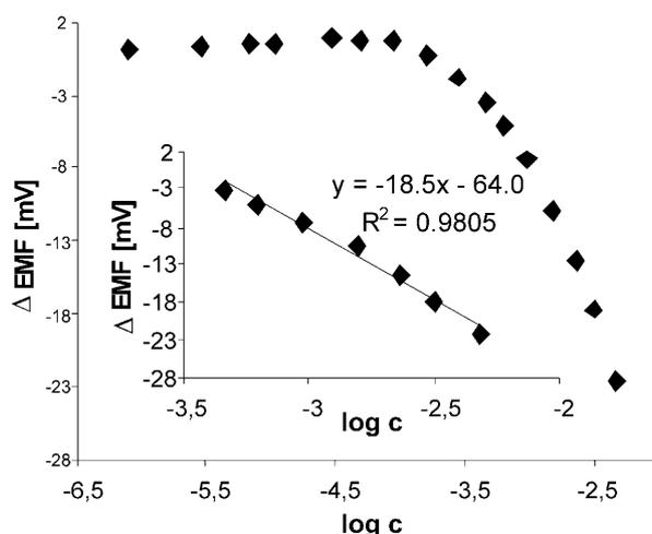
Fig. 4. Potentiometric response of the Mn(III)-porphyrin-CPE toward paracetamol. The measurements were performed in the presence of 0.01 M phosphate buffer, 0.09% NaCl, 0.5% BSA; pH 5.5 ( $n=8$ ;  $0.23 < SD < 4.2$ ).
