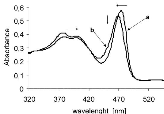
Fig. 5. UV-vis spectra of a thin PVC film doped with Mn(III)-porphyrin 1 upon exposure to paracetamol at the following concentrations: a) 0 M; b)  $1.0 \times 10^{-3}$  M. The measurements were performed in the presence of 0.01 M phosphate buffer, pH 5.5.
