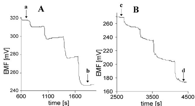
Fig. 3. Dynamic responses of Mn(III)-porphyrin ISE (A) Mn(III)-porphyrin-CPE (B). The analyte concentration was changed from a)  $3.2 \times 10^{-5}$  M to b)  $3.2 \times 10^{-3}$  M (A) and from c)  $3.2 \times 10^{-5}$  M to d)  $2.0 \times 10^{-5}$  M (B).
