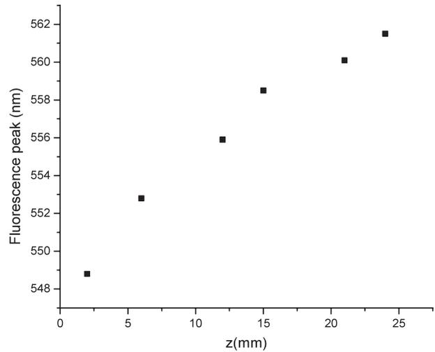
**Figure 4.** The variation of the fluorescence peak with propagation distance.
