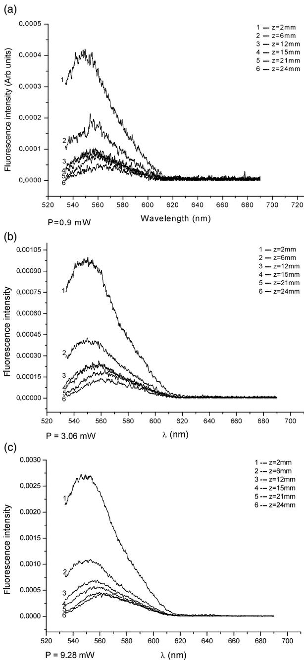
**Figure 3.** Transmitted fluorescence as a function of propagation distance through the waveguide.
