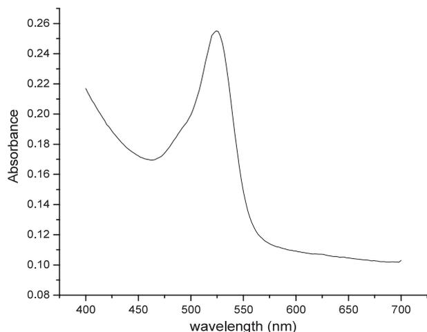
**Figure 1.** The absorption spectrum of Rh6G doped PMMA bulk sample.
