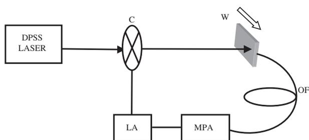
**Figure 2.** The experimental set-up used to record the fluorescence emitted from the side illuminated planar waveguide. C—chopper; W—waveguide; OF—optical fibre; LA—lock-in amplifier; MPA—monochromator–PMT assembly. The arrow shows the direction of translation of the waveguide.
