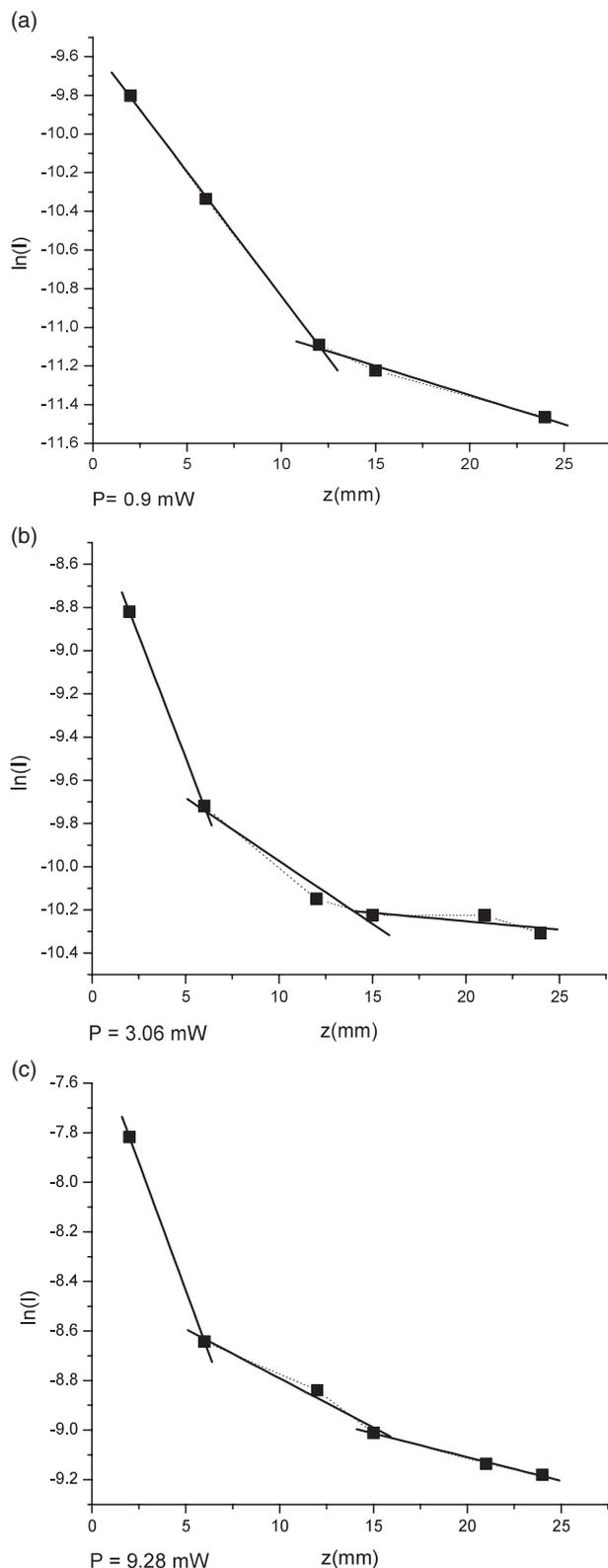
**Figure 6.** The ‘peeling the curve’ method applied to  $\ln(I)$  versus  $z$  plot at  $\lambda = 600$  nm. The solid lines represent the linear fits to the data.
