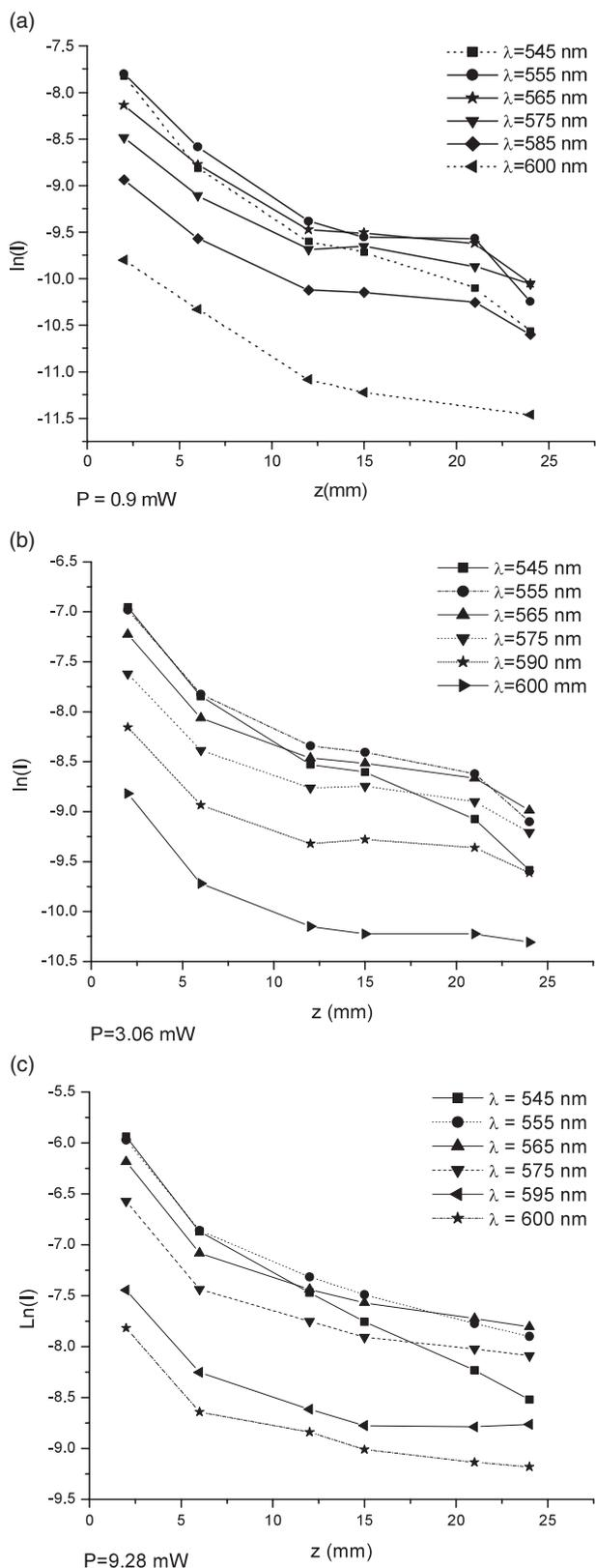
**Figure 5.** Plot of  $\ln(I)$  versus  $z$  ( $z$  is the propagation distance through the waveguide).
