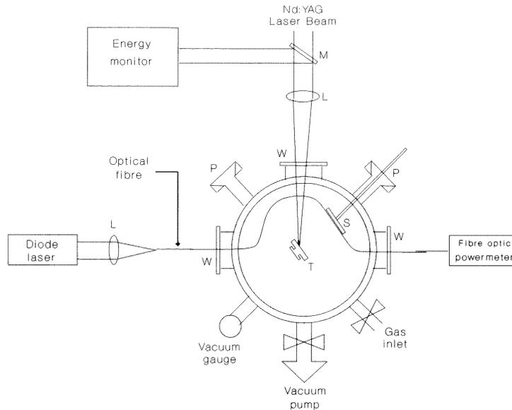
**Figure 1.** Block diagram of the experimental set-up. M, 10% reflector; L, lens; W, glass window; P, substrate insertion port; T, rotating target holder; S, glass substrate.
