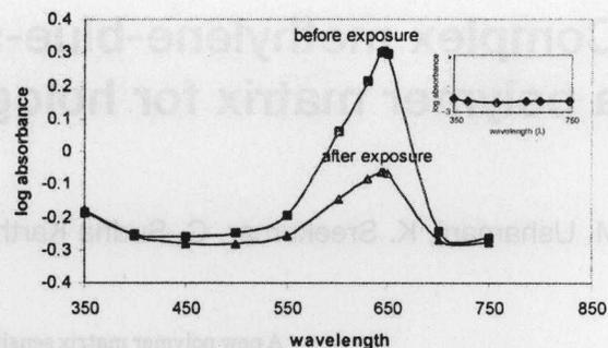
Fig. 1. Optical absorption spectra of undoped PVC (inset). CMBPVC before and after exposure are shown.
