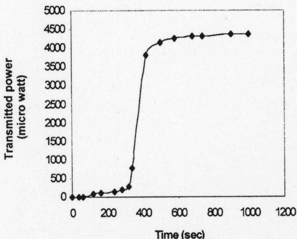
Fig. 10. Variation of transmittance as a function of recording time for an optimized sample [plot of time (s) versus transmitted power (mW)].
