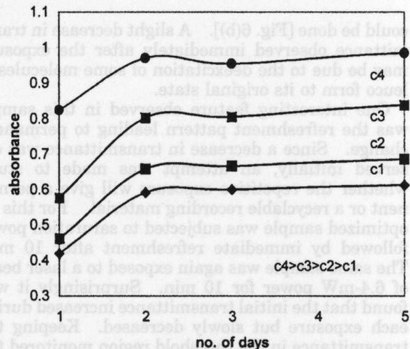
Fig. 5. Change in absorption at the irradiated spot with time for different dye concentrations (c).
