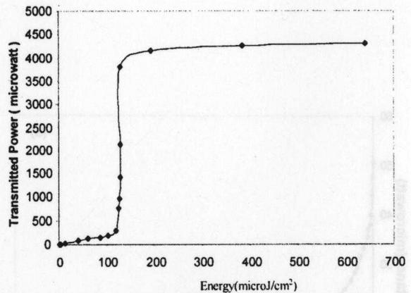
Fig. 4. Saturation energy of the sample [plot of energy ( $10^3$ ) mJ/cm<sup>2</sup> versus transmitted power (mW)].
