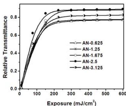
Fig. 4.1.13 Relative transmittance with exposure for MBPVA/AN films
