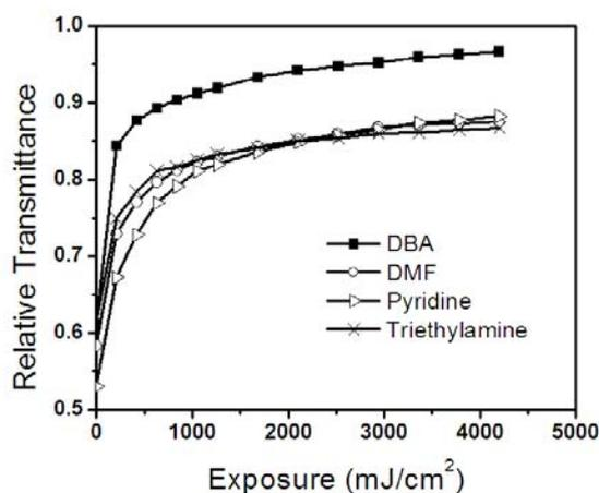
Fig.3.4 The relative transmittance of MBPVC<sub>2</sub> films with different electron donors
