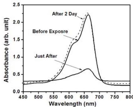
Fig. 4.1.11 The absorption spectra of MBPVA/BA film on storage.
