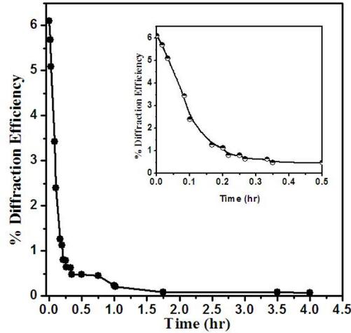
Fig. 4.2.8 The decrease in diffraction efficiency with time
