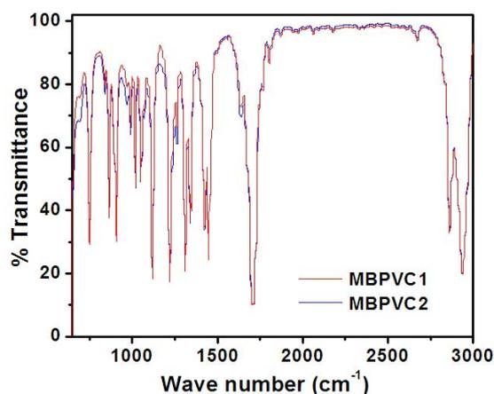
Fig. 3.3 FTIR spectra of both MBPVC<sub>1</sub> and MBPVC<sub>2</sub> solution
