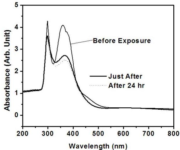
Fig. 6.16. Absorption spectra of DCPVA/AAm on laser exposure (2000mJ/cm<sup>2</sup>)
