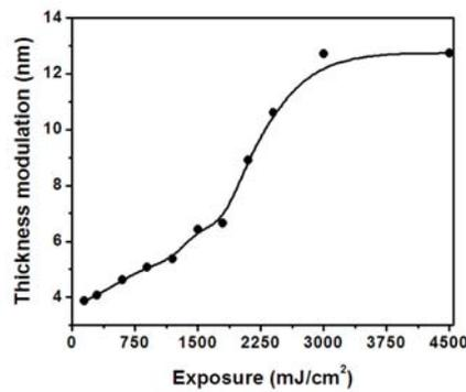
Fig. 5.15 The thickness modulation at different exposure
