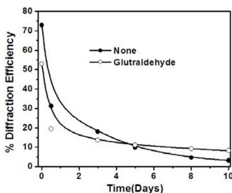
Fig.6.1 DE of both undoped and GA doped MBPVA/AAm films on storage.
