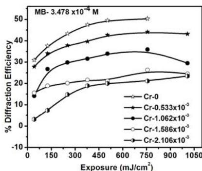
Fig.6.8 Diffraction efficiency of films having  $3.5 \times 10^{-4}$  M methylene blue
