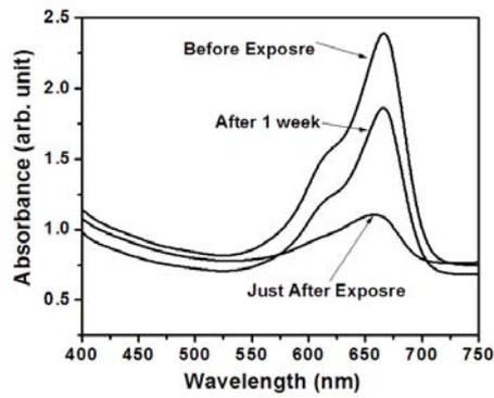
Fig. 4.1.8 The absorption spectra of MBPVA/MAA film on storage
