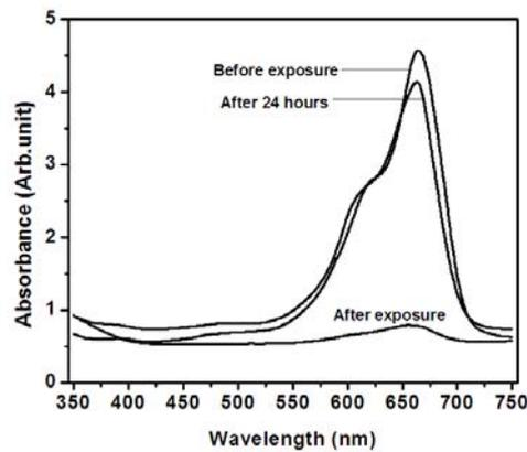
Fig. 4.1.28 The Absorption spectra of MBPVA/VAc on storage
