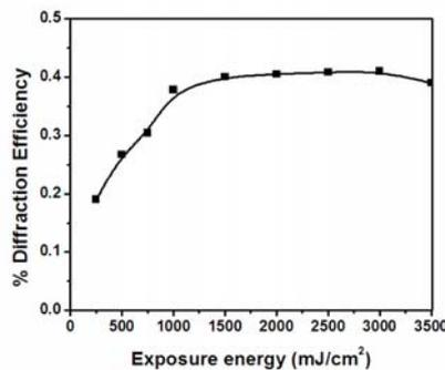
Fig. 3.13 Diffraction efficiency of P<sub>1</sub> films at different exposures
