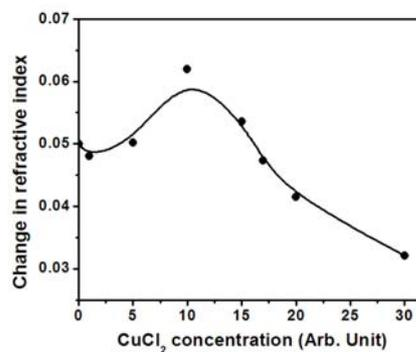
Fig.7.4 Change in refractive index for different Cu doped samples
