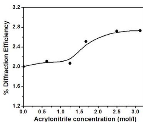
Fig. 4.1.16 The variation of DE with AN for a spatial frequency of 120 lines/mm
