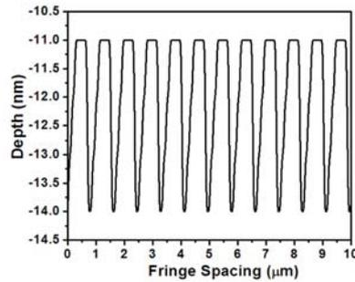
Fig. 7.9 Surface profile of the grating with a spatial frequency of 1200 lines/mm.
