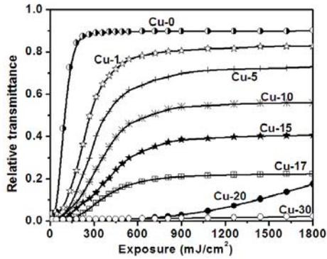
Fig. 7.1 Relative transmittance of undoped and Cu doped films at different exposures
