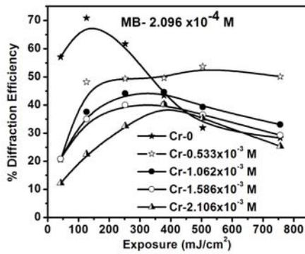
Fig.6.6 Diffraction efficiency of films having  $2.1 \times 10^{-4}$  M methylene blue
