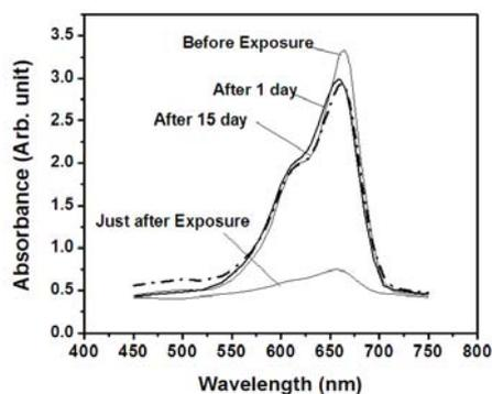
Fig.4.1.3 The absorption spectra of MBPVA/TEA film on storage
