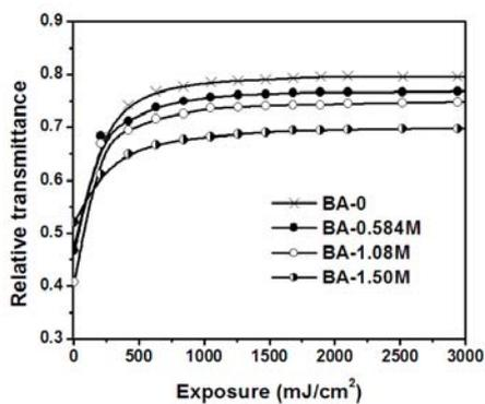
Fig. 3.15 Relative transmittance of films with different butyl acrylate concentration
