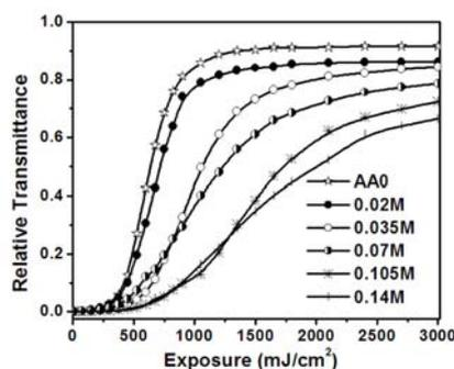
Fig.4.3.1 Relative transmittance of MBPVA/VAc films with different acrylic acid content
