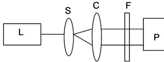
Fig.2.1 Experimental setup for real time transmittance measurements. L-Laser, S-Spatial Frequency Filter, C-Collimating lens, F-Film, P-Power meter
