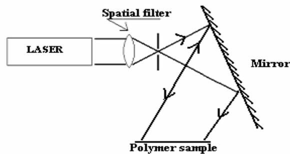
Fig. 2.3 Experimental setup to record long period gratings (single beam technique)
