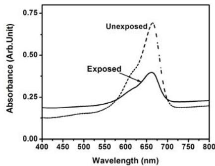
Fig.5.6 The absorption spectra of  $C_1$  film
