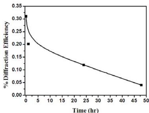
Fig.3.27. Diffraction efficiency on storage
