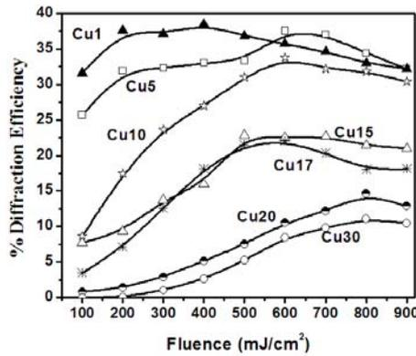
Fig.7.3 Variation of DE with copper chloride concentration.
