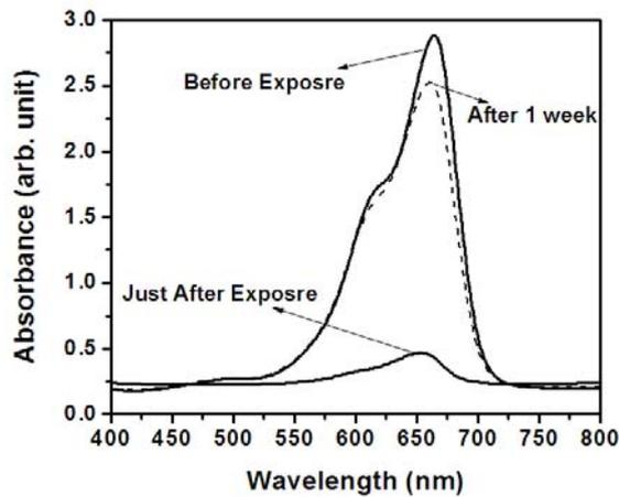
Fig. 4.1.15 The Absorption spectra of MBPVA/AN on storage.
