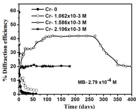
Fig.6.10. DE of both undoped and chromium doped films on storage (MB-  $2.79 \times 10^{-4}$  M)
