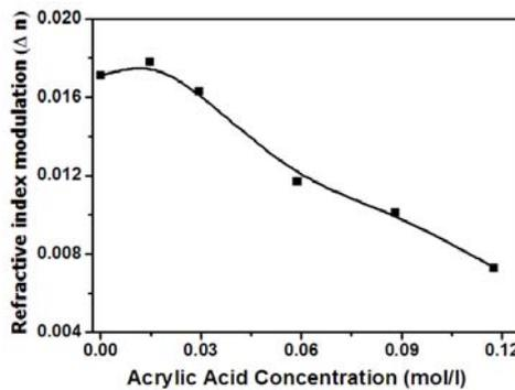
Fig. 4.3.3 Refractive index modulation on laser exposure (MBPVA/VAc)
