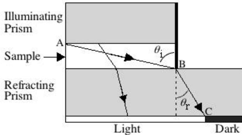
Fig.2. 2 Cross section of part of the optical path of an Abbe refractometer
