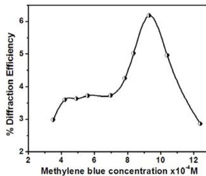
Fig. 4.2.4 Diffraction efficiency with MB concentration
