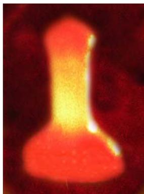
Fig.6.15. The photograph of the hologram recorded on MBDCPVA/AAm film
