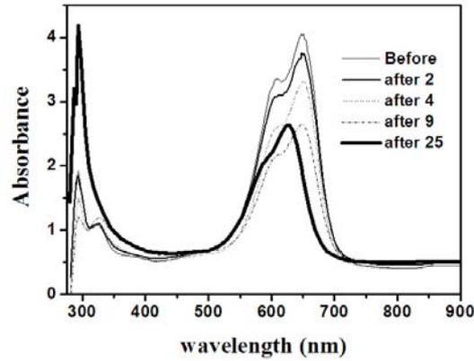
Fig. 4.2.12 Absorption spectra on reusing the sample
