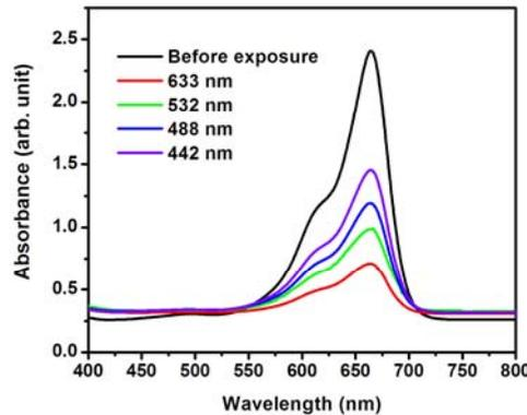
Fig. 5.30 The optical absorption spectra of the polymer film before and after exposing to different wavelengths.
