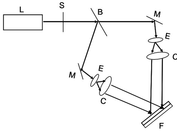
Fig. 2.3 Experimental setup to record gratings – double beam interferometry; where L-Laser, S-Shutter, B-Beam splitter, M-Mirror, E-Beam expander with spatial filter, C-Collimating lens, F-Polymer film coated on glass
