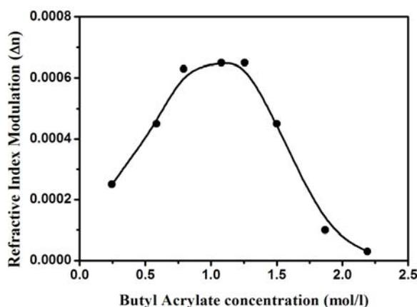
Fig. 3.18. The refractive index modulation of MBPVC/BA films on laser exposure
