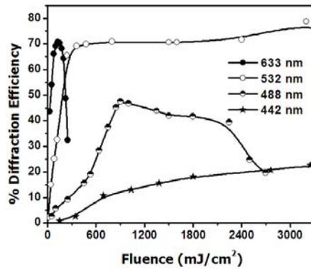
Fig. 5.31 Variation of DE with recording fluence using four different wavelengths
