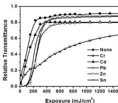
Fig. 6.2 Relative transmittance of different metal ion doped films
