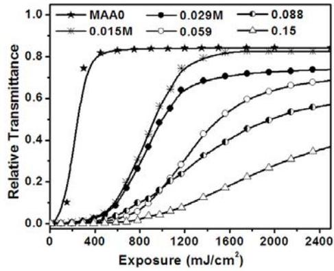
Fig. 4.1.7 Relative transmittance Vs exposure for different MBPVA/MAA films
