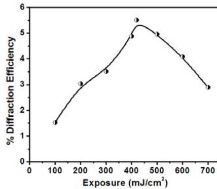
Fig. 4.1.27 The variation of diffraction efficiency with exposure
