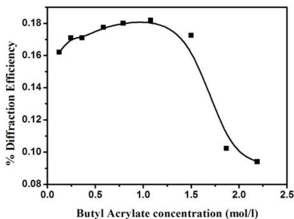
Fig. 3.17 The variation of diffraction efficiency with BA concentration.
