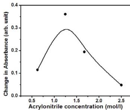
Fig. 4.1.14 The change in absorbance on laser exposure
