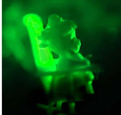
Fig.5.29 The photograph of the hologram recorded using He-Ne laser and reconstructed using Freq. doubled Nd:YAG laser
