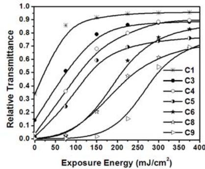
Fig. 5.5 Relative transmittance Vs exposure energy for samples with different MB
