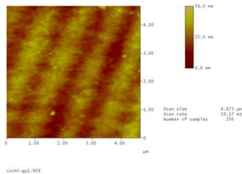
Fig. 7.8 AFM image of the gratings recorded with 1100 lines/mm (2D view)
