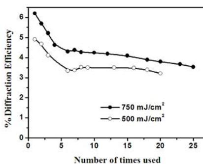
Fig. 4.2.14 Diffraction efficiency on reusing of the sample (MBPVA/VAc/ethanol)
