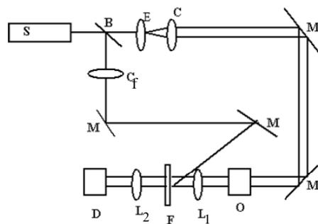
Fig.2.5 The experimental technique used for recording FT hologram. where S-Laser, B-beam splitter, E-beam expander with spatial filter, C-Collimating lens, M-Mirror, O-object (transparency),  $L_1$  and  $L_2$ -Lens,  $C_f$ -Focusing lens, F-Polymer film, D-CCD
