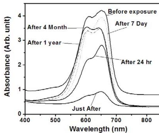
Fig. 4.3.7. The absorption spectra of MBPVA/VAc/MAA film on storage
