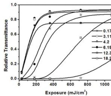
Fig. 4.1.23 The relative transmittance with different MB concentration
