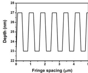
Fig. 5.23 The surface mapping of the gratings recorded with 1600 lines/mm
