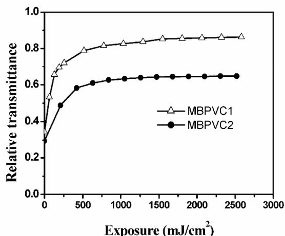
Fig. 3.2 Relative transmittance of MBPVC films prepared by two different procedures.
