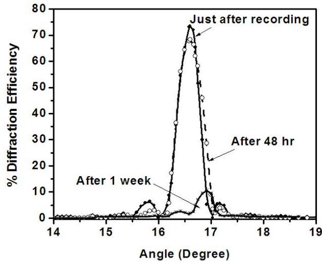
Fig.5.24 The angular response of MBPVA/AAm on storage
