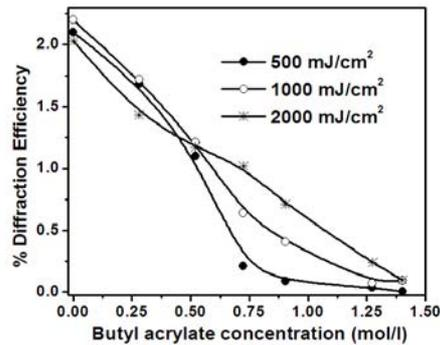
Fig. 4.1.12 The variation of diffraction efficiency with BA concentration
