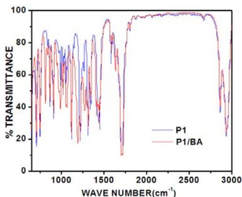
Fig. 3.14 FTIR spectrum of P<sub>1</sub> and butyl acrylate doped P<sub>1</sub> samples
