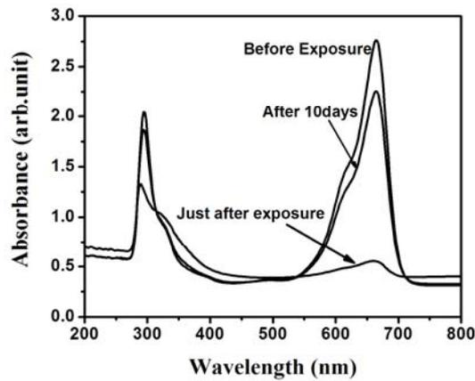
Fig. 5.17 The absorption spectra on storage
