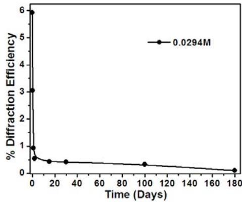
Fig. 4.3.10. The efficiency of MBPVA/VAc/MAA film on storage (MAA= 0.029M)
