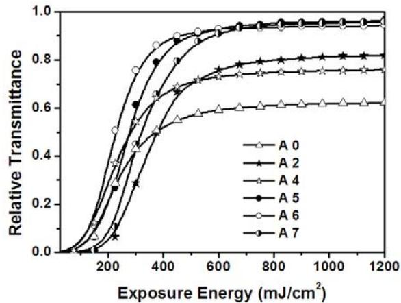
Fig. 5.1 Real time transmittance of films with different AAm concentration
