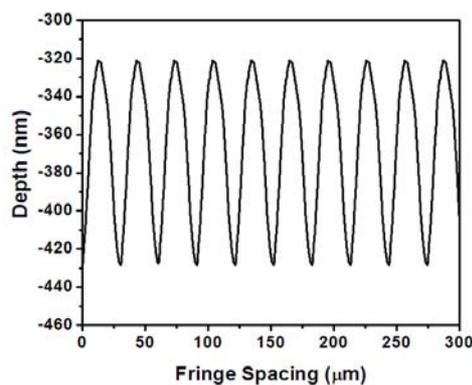
Fig.4.3.11 The surface profile of gratings recorded on MBPVA/VAc/MMA film
