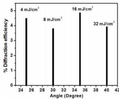
Fig. 5.26 The diffraction efficiency of gratings multiplexed to have equal efficiency
