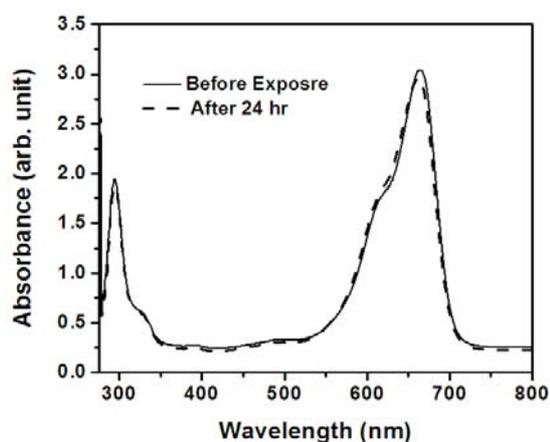
Fig. 4.2.10 The absorption spectra of MBPVA/VAc before and after irradiation
