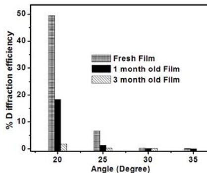
Fig. 5.25. The efficiency of gratings multiplexed with an exposure of  $50\text{mJ}/\text{cm}^2$
