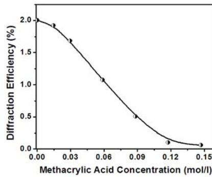
Fig. 4.1.9 The variation of diffraction efficiency with MAA
