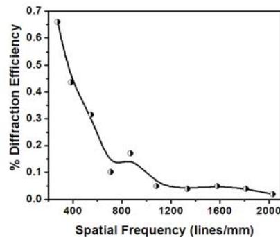
Fig. 4.2.15 Variation of diffraction efficiency with spatial frequency.
