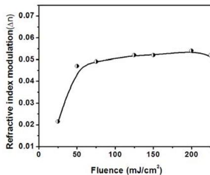
Fig. 5.13 The variation of refractive index modulation with exposure
