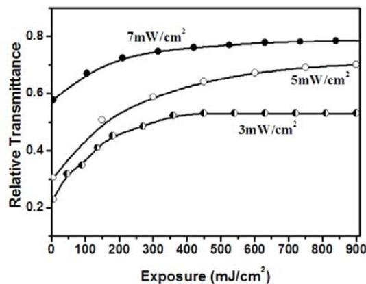
Fig. 3.20 The relative transmittance of MBPVA/BA film for different input powers
