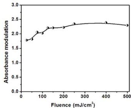
Fig. 5.12 The variation of absorbance modulation with exposure
