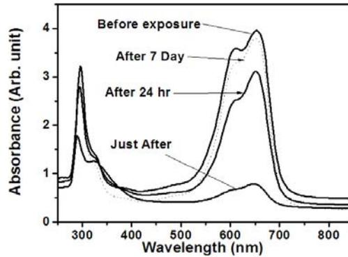
Fig. 4.3.2. The absorption spectra of MBPVA/VAc film with 0.035M acrylic acid.
