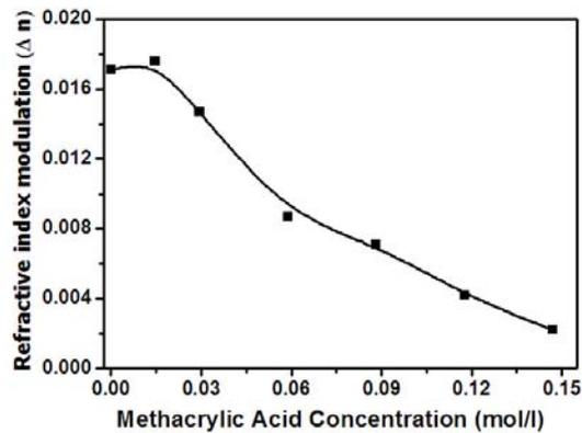
Fig. 4.3.8. The refractive index modulation on laser exposure
