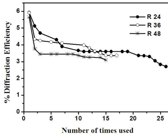
Fig. 4.2.11 Diffraction efficiency on reusing of the sample (optimum composition)
