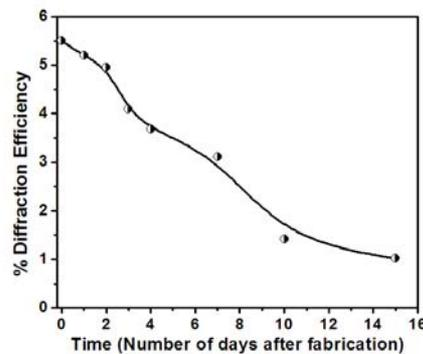
Fig. 4.1.29 The efficiency on ageing of the film
