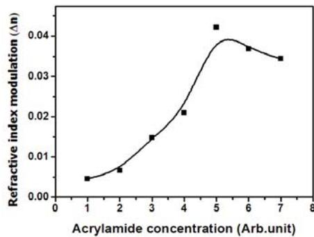
Fig.5. 3 The refractive index modulation arises on laser exposure
