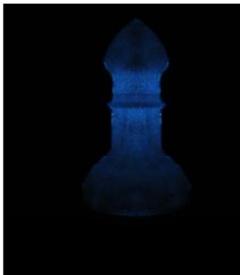
Fig. 6.19 Photograph of the hologram recorded on DCPVA/AAM
