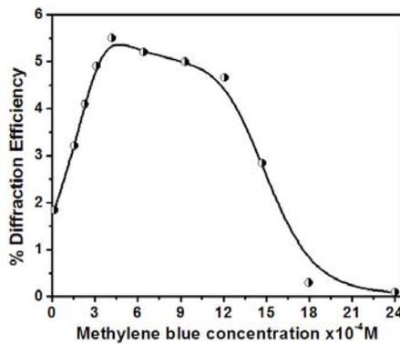
Fig. 4.1.25 The variation of diffraction efficiency with dye concentration
