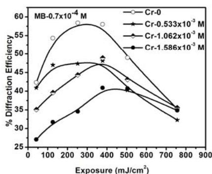
Fig.6.4 Diffraction efficiency of films having  $0.7 \times 10^{-4}$  M methylene blue
