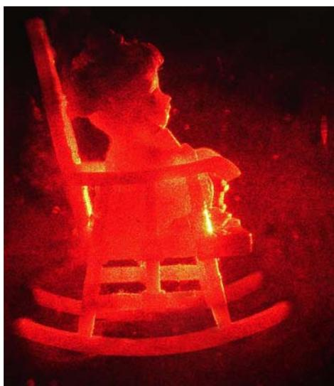
Fig.5.28 The photograph of the hologram recorded and reconstructed using He-Ne laser
