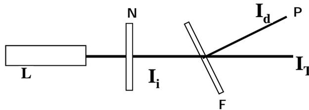
Fig. 2.4 Experimental setup for diffraction efficiency measurements.
