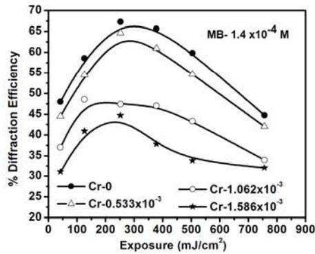
Fig.6.5 Diffraction efficiency of films having  $1.4 \times 10^{-4}$  M methylene blue
