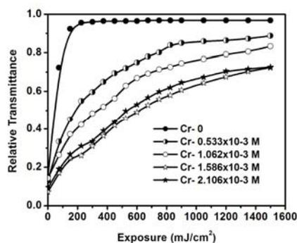
Fig.6.13. Relative transmittance of both undoped and Cr doped films (MB-  $2.79 \times 10^{-4}\text{M}$ )
