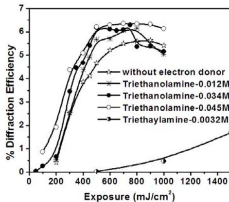
Fig. 4.2.7 The diffraction efficiency obtained for different electron donors
