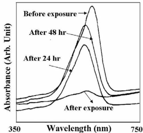
Fig. 4.1.2 The absorption spectra of MBPVA film on storage.
