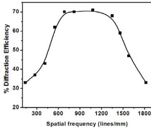
Fig. 5.21 The variation of diffraction efficiency with spatial frequency
