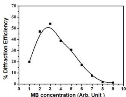
Fig. 5.9 The variation of diffraction efficiency with MB concentration
