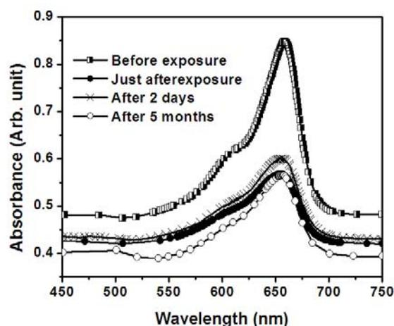
Fig.3.23 Absorption spectra of MBPVC/VAc films on storage
