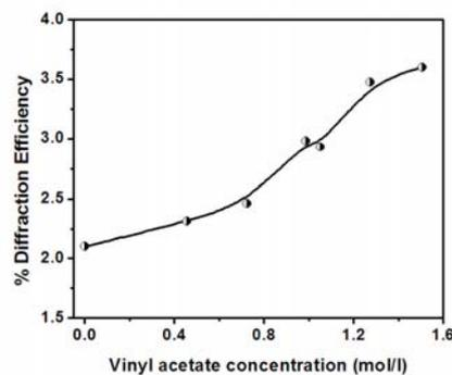
Fig. 4.2.2 Variation of Diffraction efficiency with VAc concentration
