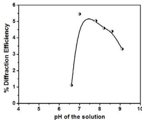
Fig. 4.1.26 The variation of diffraction efficiency with pH
