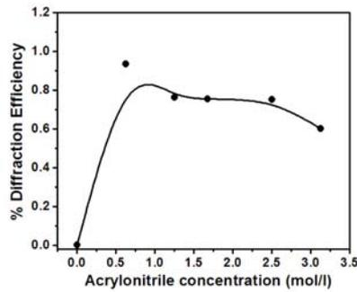
Fig. 4.1.17 The diffraction efficiency on storage (3 days after grating formation)
