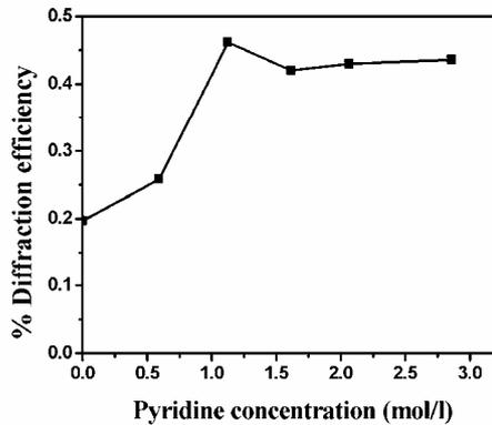
Figure 3.9 Variation of diffraction efficiency with pyridine concentration
