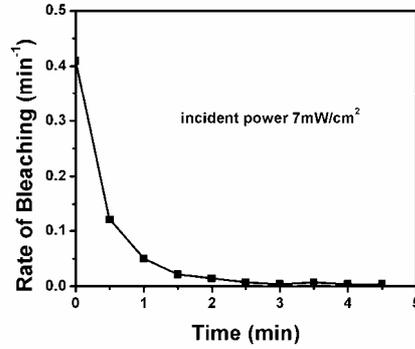
Fig. 3.8 Rate of bleaching of sample with pyridine concentration 1.126 M (sample P<sub>1</sub>)
