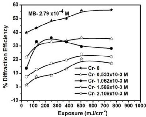
Fig.6.7 Diffraction efficiency of films having  $2.79 \times 10^{-4}$  M methylene blue
