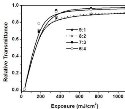
Fig. 4.1.19. The relative transmittance of films with different PVA/VAc ratio
