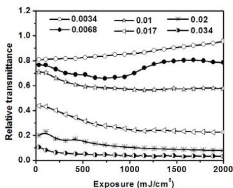
Fig. 6.17 The relative transmittance of DCPVA/ADC films
