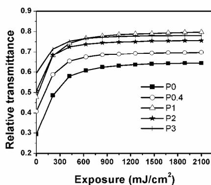
Fig. 3.7. Relative transmittance of samples with different pyridine concentrations
