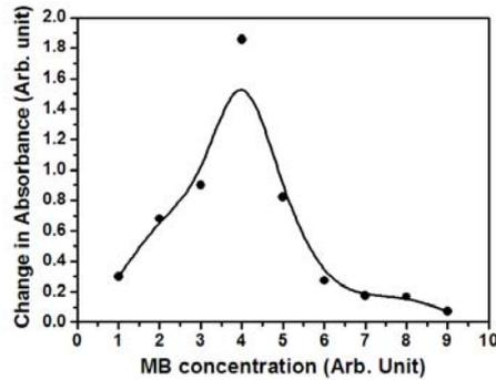
Fig. 5.7 Absorbance modulation on laser exposure for films with different MB concentration
