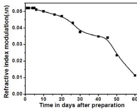
Fig. 5.20 The refractive index modulation on ageing of the film
