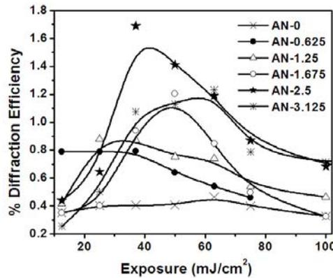
Fig. 4.1.18 DE with exposure for different AN concentration. (spatial frequency=300 lines/mm)
