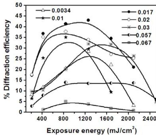
Fig. 6.18. Diffraction efficiency of DCPVA/AAM films
