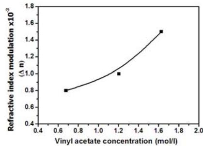
Fig. 4.1.22 The variation of change in refractive index on laser exposure
