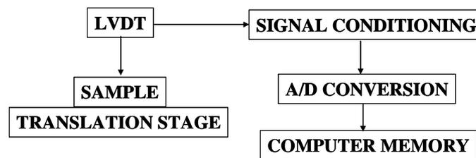
Figure 2.7 Block Diagram of Stylus Profiler
