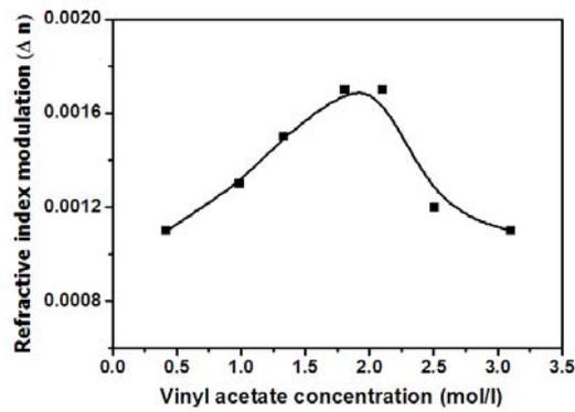
Fig.3.25. Refractive index modulation on laser exposure
