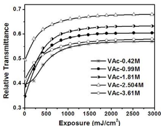
Fig.3.22 Relative transmittance of MBPVC/VAc films at different exposure
