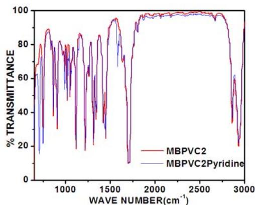
Fig. 3.6 FTIR spectra of both undoped and pyridine doped samples (P<sub>1</sub>)
