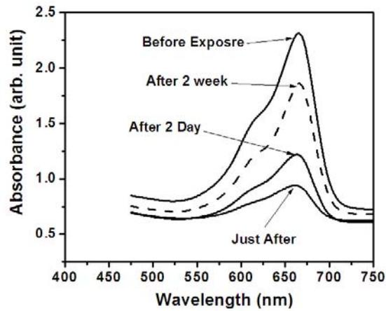
Fig. 4.1.5 The absorption spectra of MBPVA/AA film on storage
