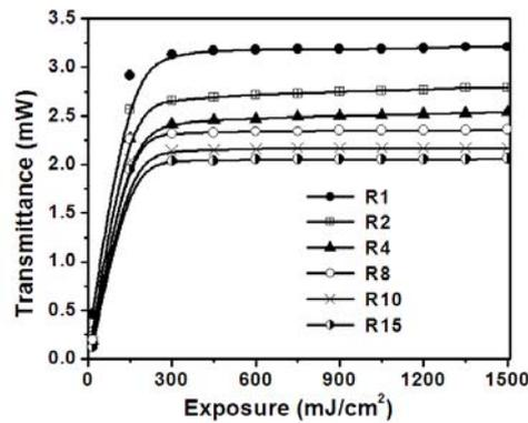
Fig. 4.2.13 Real time transmittance on reusing the sample
