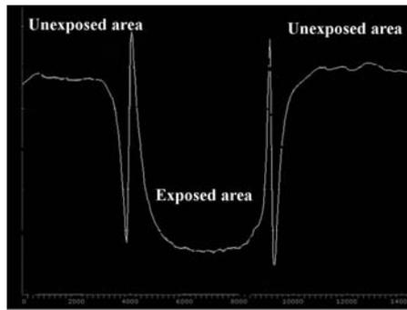
Fig. 5.14 The surface profile of MBPVA/AAm film on uniform illumination
