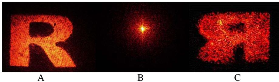
Fig.7.15. FT hologram of letter 'R' recorded on Cu doped film where (A) is the object, (B) FT and (C) the reconstructed image.
