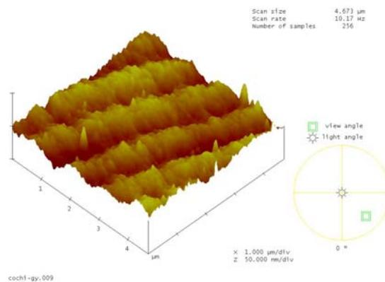
Fig. 7.7 AFM image of the gratings recorded with 1100 lines/mm (3D view)
