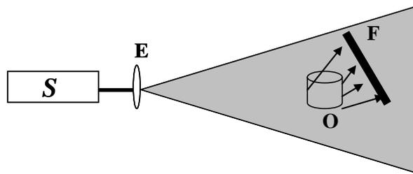
Fig.2. 6 The experimental technique used for recording transmission hologram. where
