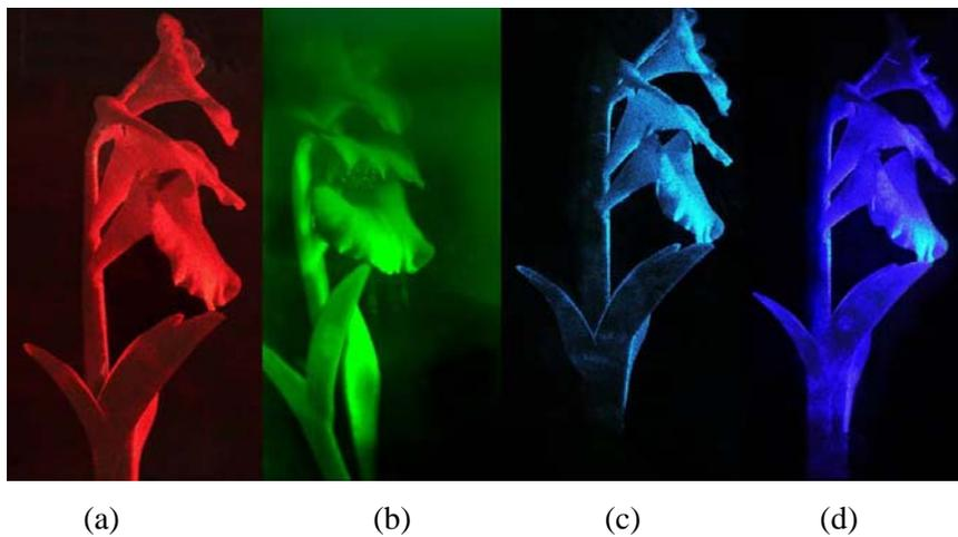
Fig. 5.32. Transmission hologram recorded using He-Ne laser (a), Nd: YAG laser (b), Ar<sup>+</sup> laser (c) and He-Cd laser (d)
