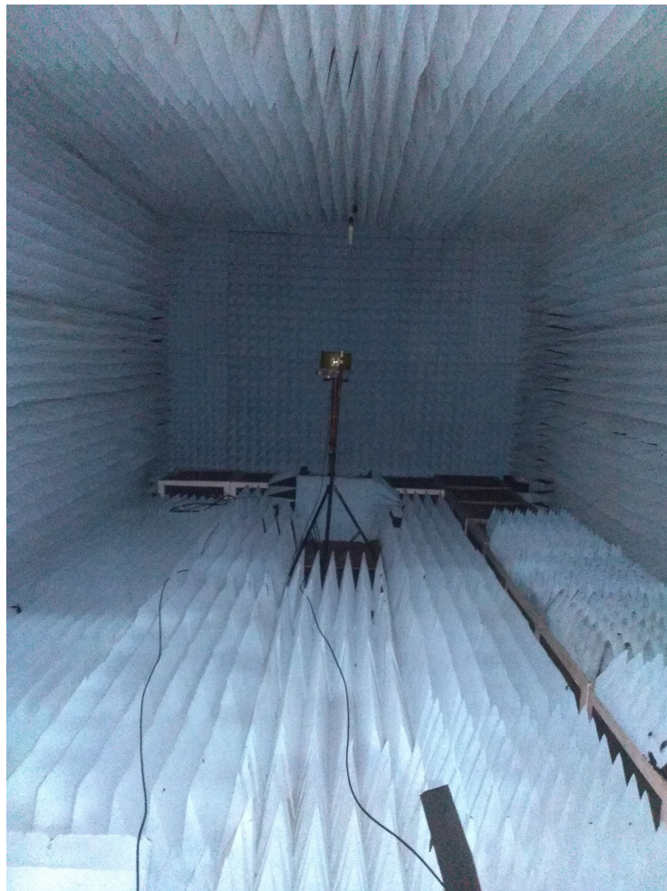
Figure 3.8: Anechoic chamber and turn table assembly.
