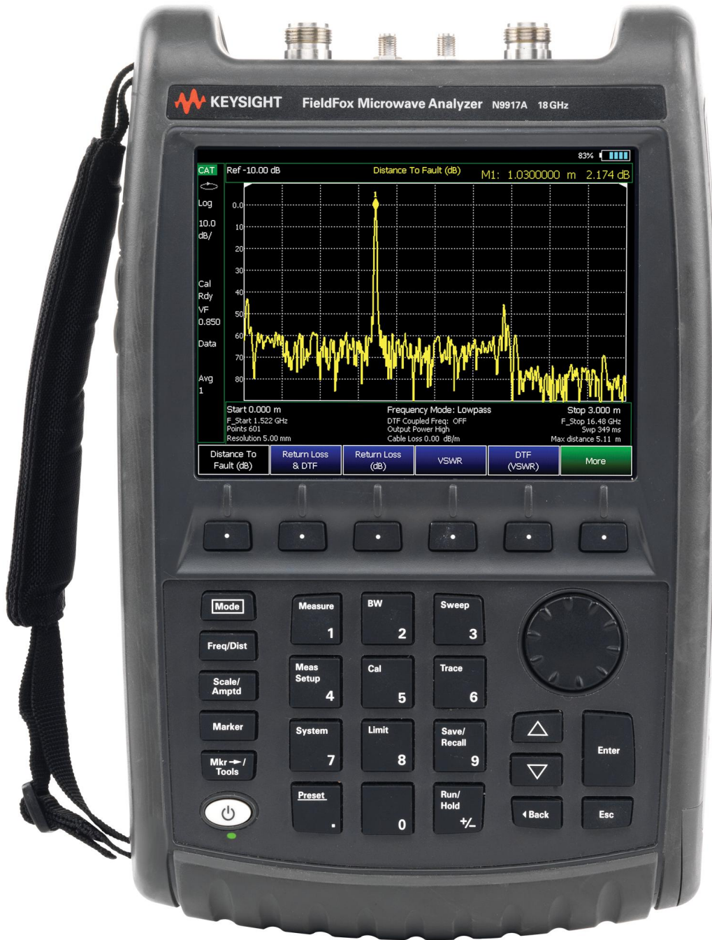
Figure 3.7: Keysight Fieldfox N9927A handheld VNA (30 kHz to 20 GHz)
