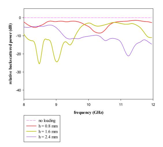
**Fig 5.6** Variation of backscattered power with frequency for the 90<sup>0</sup> dihedral corner loaded with dielectric backed second iterated SCF array of different dielectric thickness (h)
