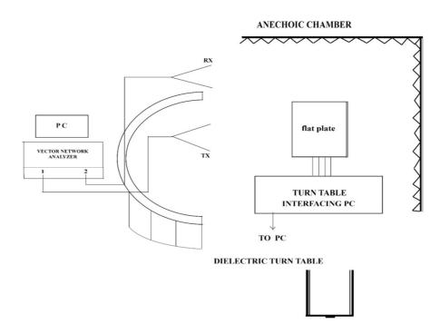
Fig 3.2 Schematic diagram of the Arch Method
