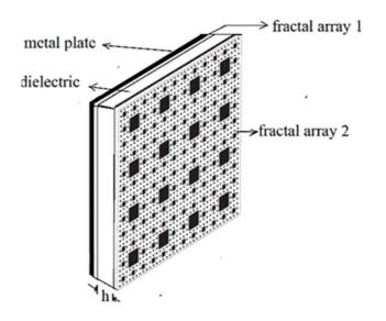
Fig 3.9 Stacked SCF arrays over flat plate
