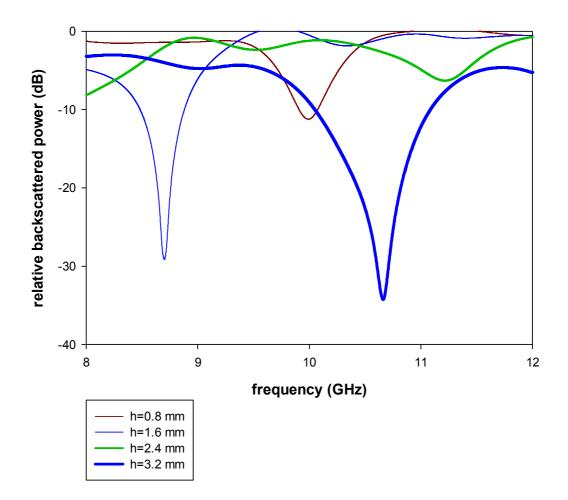
Fig 4.24 Variation of relative backscattered power with frequency for the fully interleaved structure
