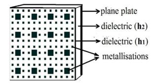
Fig. 4.12 Schematic diagram of the dielectric backed 4×4 SCF array
