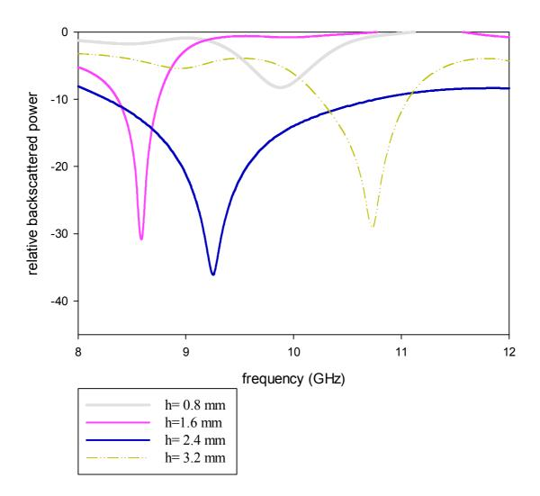
Fig 4.26 Variation of relative backscattered power with frequency when loaded with horizontal interleaved structure
