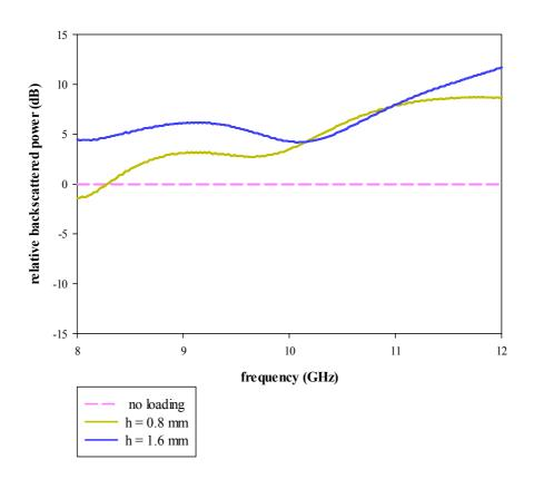
**Fig 6.13** Measured variation of relative backscattered power with frequency for 110<sup>0</sup> wedge loaded with third iterated SCF array
