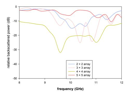
Fig 4.2 Variation of relative backscatterd power with frequency for second iterated stage SCF array for different combinations
