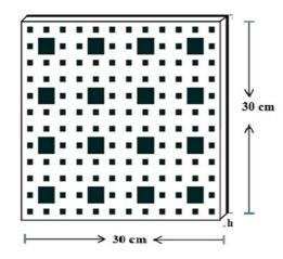
**Fig 4.4** Schematic diagram of Flat metal plate loaded with SCF array backed with dielectric
