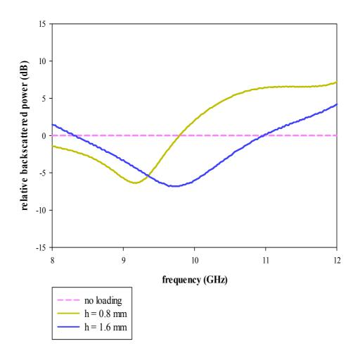
**Fig 6.15** Measured variation of relative backscattered power with frequency for 120<sup>0</sup> wedge loaded with second iterated SCF array
