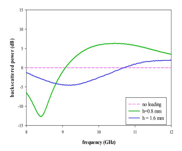
**Fig 6.9** Measured variation of relative backscattered power with frequency for 100<sup>0</sup> wedge loaded with second iterated SCF array
