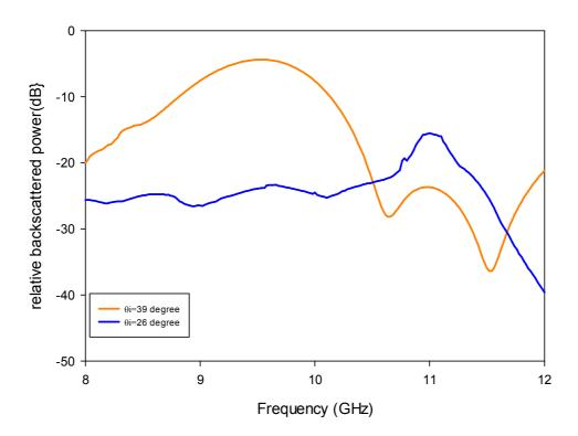
**Fig.4.16** Relative backscattered power with frequency at angle of incidence  $\theta_i=39^0$  and  $\theta_i=26^0$  for the second iterated stage of SCF array. (h<sub>1</sub>=0.8mm & h<sub>2</sub>=4.5mm)
