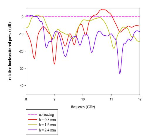
**Fig 5.3** Variation of backscattered power with frequency for the 80<sup>0</sup> dihedral corner loaded with dielectric backed second iterated SCF array of different dielectric thickness (h)
