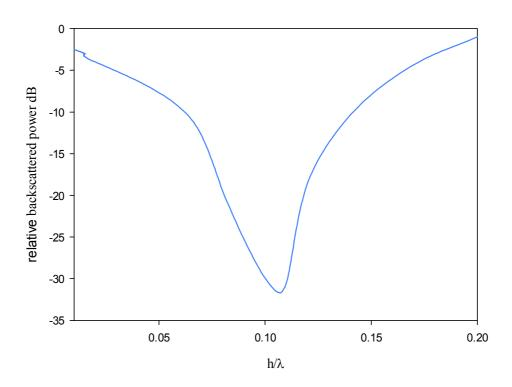
Fig 4.11 Variation of relative backscattered power with dielectric thickness for second iterated stage of the SCF array for frequency of 11.08
