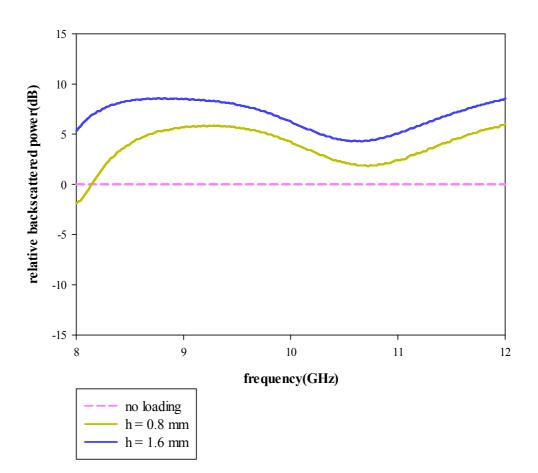
**Fig 6.7** Measured variation of relative backscattered power with frequency for 90<sup>0</sup> wedge loaded with third iterated SCF array
