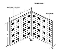
Fig 5.1 Schematic diagram of the dihedral corner reflector loaded with second iterated stage of the SCF array
