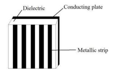
Fig 1.5 Schematic diagram of a strip grating
