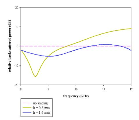
**Fig 6.12** Measured variation of relative backscattered power with frequency for 110<sup>0</sup> wedge loaded with second iterated SCF array
