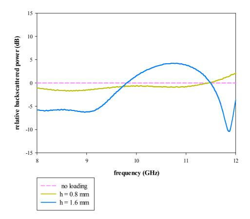
**Fig 6.14** Measured variation of relative backscattered power with frequency for 120<sup>0</sup> wedge loaded with first iterated SCF array
