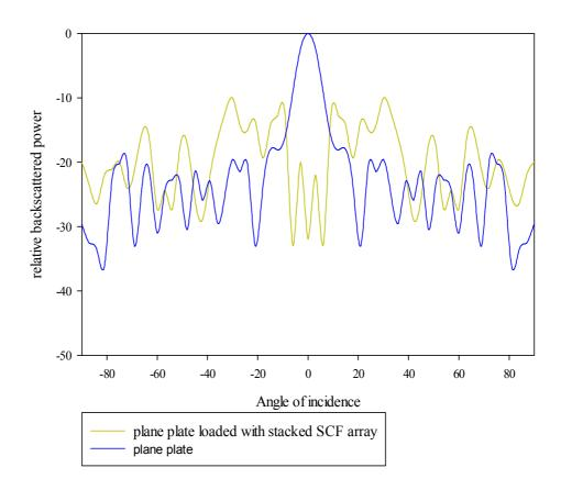
**Fig 4.21** Variation of relative backscattered power with angle of incidence at f=11.08 GHz for stacked SCF array
