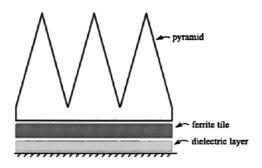
Fig 3.1 Pyramidal absorbers in the wall of an anechoic chamber
