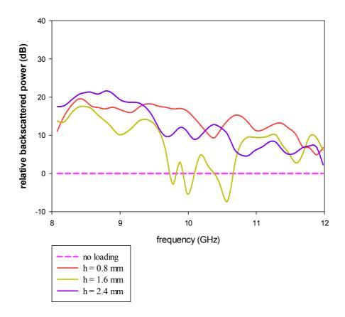
**Fig 5.9** Variation of backscattered power with frequency for the 100<sup>0</sup> dihedral corner loaded with dielectric backed first iterated SCF array of different dielectric thickness (h)
