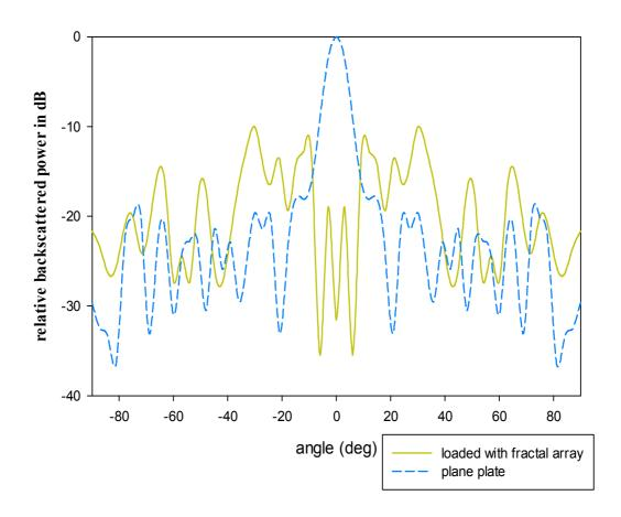
**Fig 4.8** Variations of relative backscattered power with angle of incidence at f=11.08 GHz for second iterated stage of SCF array and thickness h=3.2mm
