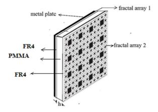
Fig. 4.18 Stacking of two different iterated stages of SCF array
