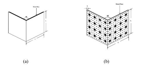
Fig 6.1 Schematic diagram of (a) plain wedge (b) wedge loaded with second iterated stage of SCF array with dielectric thickness (h) with wedge angle  $\alpha$
