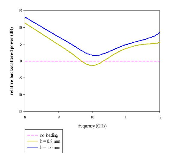
**Fig 6.4** Measured variation of relative backscattered power with frequency for 80<sup>°</sup> wedge loaded with third iterated SCF array
