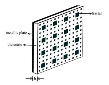
Fig 3.8 Flat metallic plate loaded with dielectric backed second stage of SCF Array
