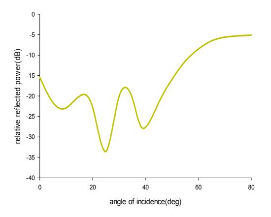
Fig.4.13 Variation of relative reflected power with angle of incidence for the SCF array at 9.8 GHz .( $h_1$ =0.8mm &  $h_2$ =4.5mm)
