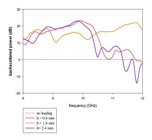
**Fig 5.10** Variation of backscattered power with frequency for the 100<sup>0</sup> dihedral corner loaded with dielectric backed second iterated SCF array of different dielectric thickness (h)
