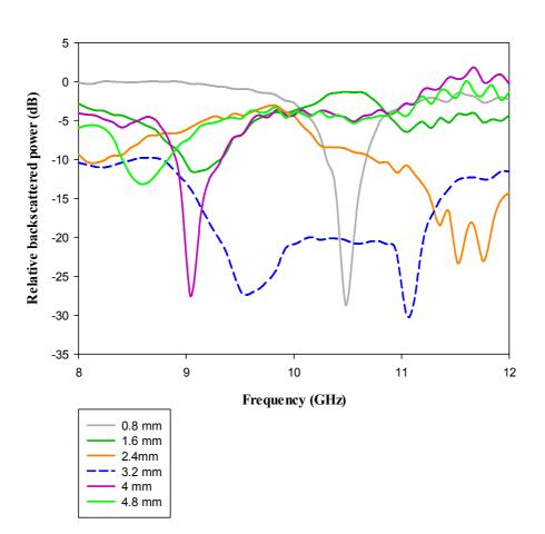
**Fig 4.5** Variations of relative backscattered power for metallic plate loaded with 2<sup>nd</sup> iterated stage of SCF array with different dielectric thickness
