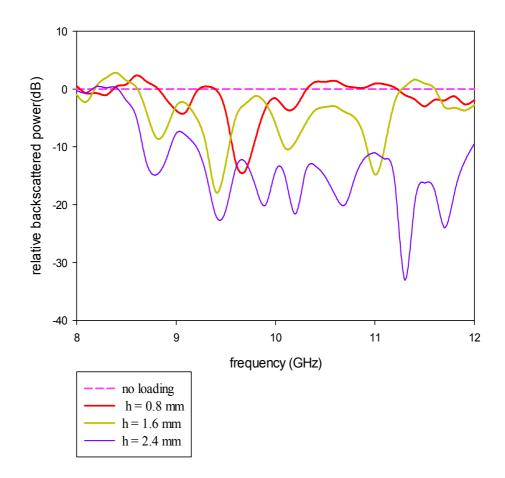
**Fig 5.4** Variation of backscattered power with frequency for the 80<sup>0</sup> dihedral corner loaded with dielectric backed third iterated SCF array of different dielectric thickness (h)
