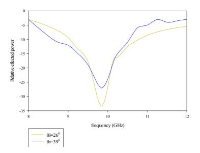
Fig.4.15 Variation of relative reflected power with frequency for the second iterated stages of the SCF arrays for  $\theta_i = 26^{0}$  and  $\theta_i = 39^{0}$ .(h<sub>1</sub>=0.8mm & h<sub>2</sub>=4.5mm)
