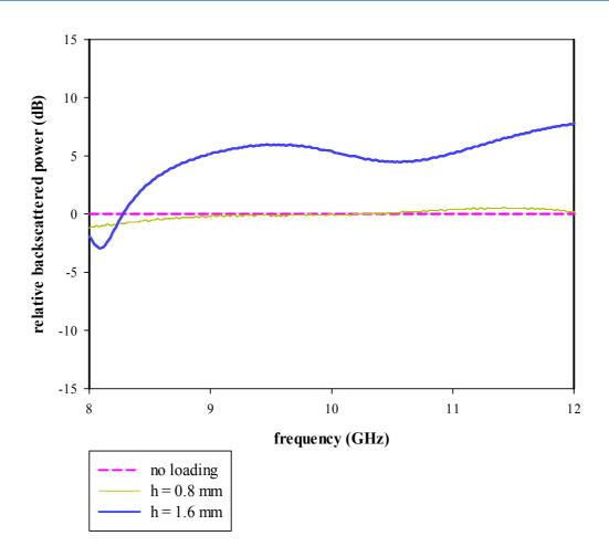
**Fig 6.5** Measured variation of relative backscattered power with frequency for 90<sup>0</sup> wedge loaded with first iterated SCF array
