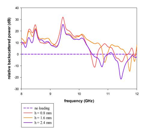
**Fig 5.11** Variation of backscattered power with frequency for the 100<sup>0</sup> dihedral corner loaded with dielectric backed third iterated SCF array of different dielectric thickness (h)
