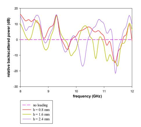
**Fig 5.12** Variation of backscattered power with frequency for the 110<sup>0</sup> dihedral corner loaded with dielectric backed first iterated SCF array of different dielectric thickness (h)
