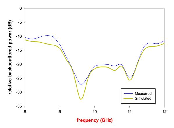
**Fig 4.7** Variation of backscattered power with frequency response for the second iterated stage of dielectric backed 4 × 4 SCF array
