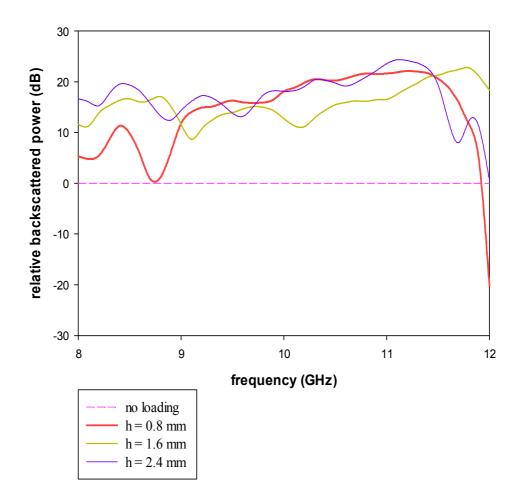
**Fig 5.13** Variation of backscattered power with frequency for the 110<sup>0</sup> dihedral corner loaded with dielectric backed second iterated SCF array of different dielectric thickness (h)
