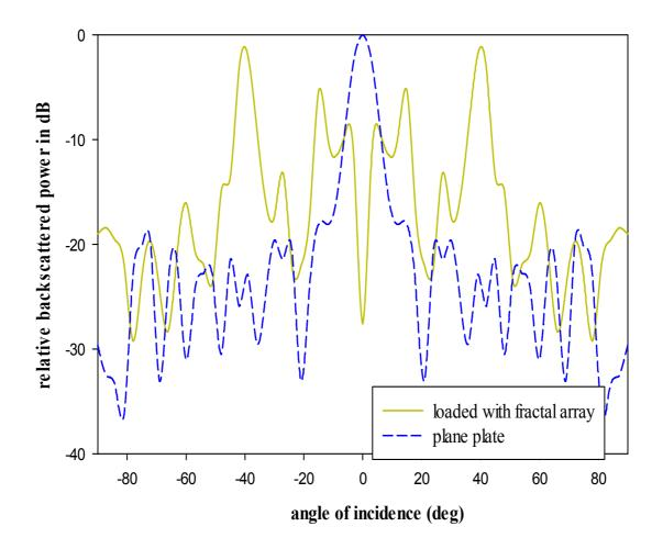
Fig 4.9 Variations of relative backscattered power with angle of incidence for frequency f=9.5 GHz for second iterated stage of SCF array (h=3.2mm.)
