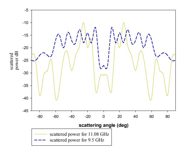
Fig 4.10 Variation of scattered power with scattering angle at 11.08 GHz and 9.5 GHz for the second iterated stage of the SCF array with thickness h=3.2mm at normal incidence
