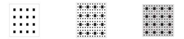
Fig 1.8  $4 \times 4$  Sierpinski carpet fractal arrays of first second and third iteration
