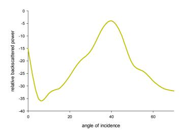
Fig 4.14 Variation of relative backscattered power with angle of incidence for the SCF array at 9.8 GHz .(h<sub>1</sub>=0.8mm & h<sub>2</sub>=4.5mm)
