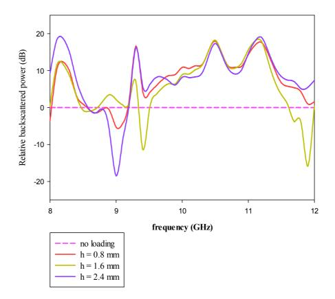
Fig 5.16 Variation of backscattered power with frequency for the second iterated stage of 120<sup>0</sup> dielectric backed SCF array
