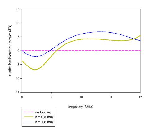
**Fig 6.16** Measured variation of relative backscattered power with frequency for 120<sup>0</sup> wedge loaded with third iterated SCF array
