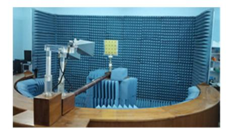
Fig 3.3 Photograph of Arch method
