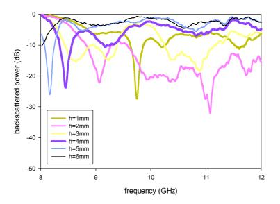
Fig 4.19 Variation of backscattered power with frequency for different dielectric thickness
