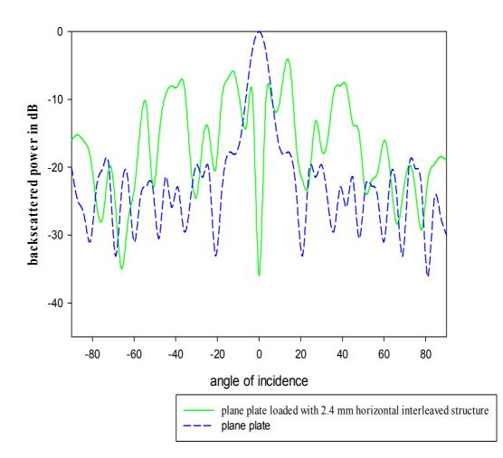
Fig 4.27 Variation of relative backscattered power with angle of incidence of the horizontally interleaved SCF array loaded over the flat plate with a dielectric thickness of 2.4 mm
