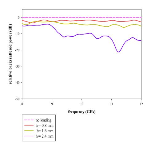
**Fig 5.5** Variation of backscattered power with frequency for the 90<sup>0</sup> dihedral corner loaded with dielectric backed first iterated SCF array of different dielectric thickness (h)
