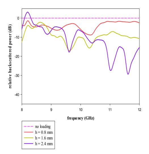
**Fig 5.7** Variation of backscattered power with frequency for the 90<sup>0</sup> dihedral corner loaded with dielectric backed third iterated SCF array of different dielectric thickness (h)
