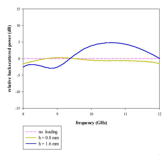
**Fig 6.8** Measured variation of relative backscattered power with frequency for 100<sup>°</sup> wedge loaded with first iterated SCF array
