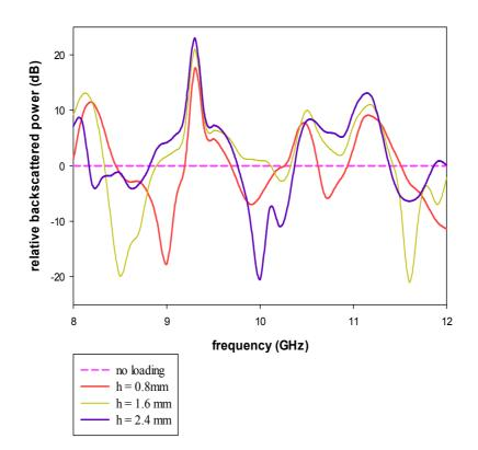
**Fig 5.15** Variation of backscattered power with frequency for the 120<sup>0</sup> dihedral corner loaded with dielectric backed first iterated SCF array of different dielectric thickness (h)
