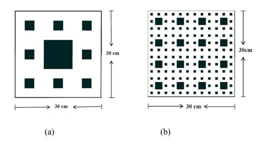
**Fig 3.6** Second iterated stage of (a) Sierpinski Carpet (b) Sierpinski Carpet Array The corresponding first and third iterations are also shown below
