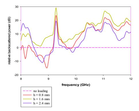
Fig 5.17 Variation of backscattered power with frequency for the third iterated stage of  $120^{\circ}$  dielectric backed SCF array
