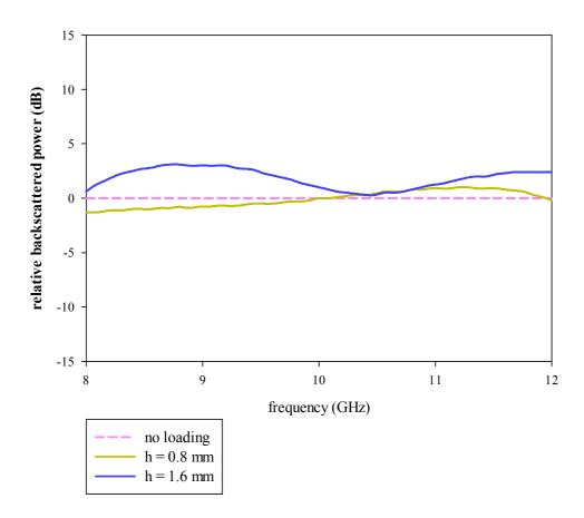
**Fig 6.2** Measured variation of relative backscattered power with frequency for 80<sup>°</sup> wedge loaded with first iterated SCF array
