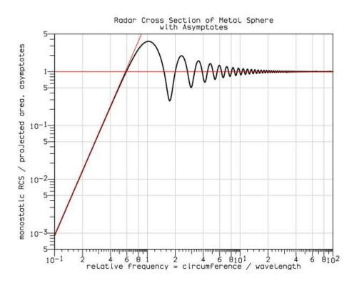
Fig 1.2 Plot of the radar cross section as a function of the electrical size of the target
