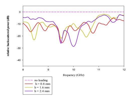
**Fig 5.2** Variation of backscattered power with frequency for the 80<sup>0</sup> dihedral corner loaded with dielectric backed first iterated SCF array of different dielectric thickness (h)
