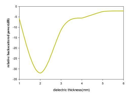
Fig 4.20 Variation of backscattered power with dielectric thickness at f=11.08 GHz
