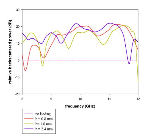
**Fig 5.14** Variation of backscattered power with frequency for the 110<sup>0</sup> dihedral corner loaded with dielectric backed third iterated SCF array of different dielectric thickness (h)
