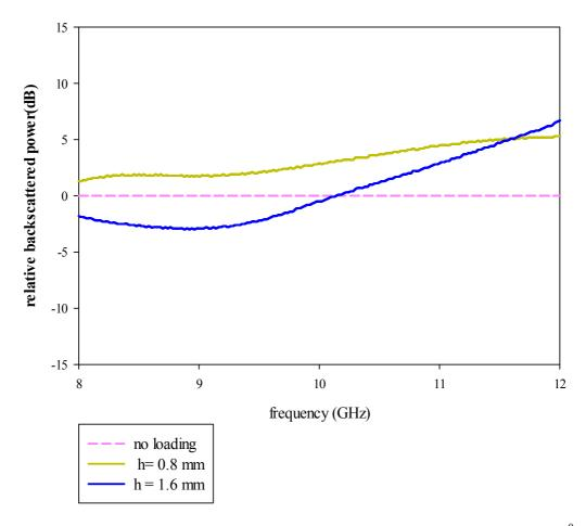
**Fig 6.3** Measured variation of relative backscattered power with frequency for 80<sup>°</sup> wedge loaded with second iterated SCF array
