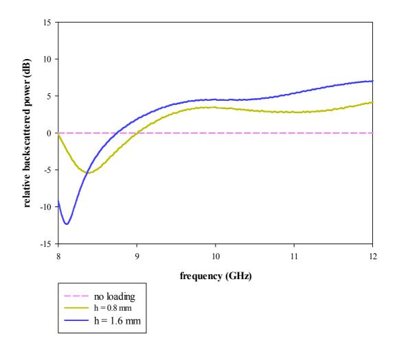
**Fig 6.6** Measured variation of relative backscattered power with frequency for 90<sup>°</sup> wedge loaded with second iterated SCF array
