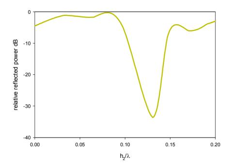
Fig.4.17 Variation of relative reflected power with dielectric thickness  $(h_2)$  for the second iterated stage of the SCF array with  $h_1=0.8$ mm
