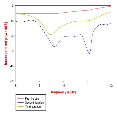
**Fig 4.6** Variation of relative backscattered power with frequency for various iterated stage of dielectric backed Sierpinski carpet array with thickness h=3.2mm
