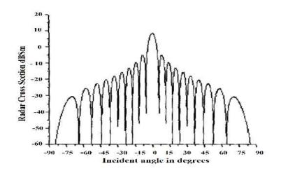
Fig 1.3 RCS pattern of a flat metal plate
