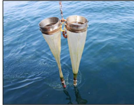
**Fig. 2.3. Sampling gear- Hydro Bios Bongo Net**
