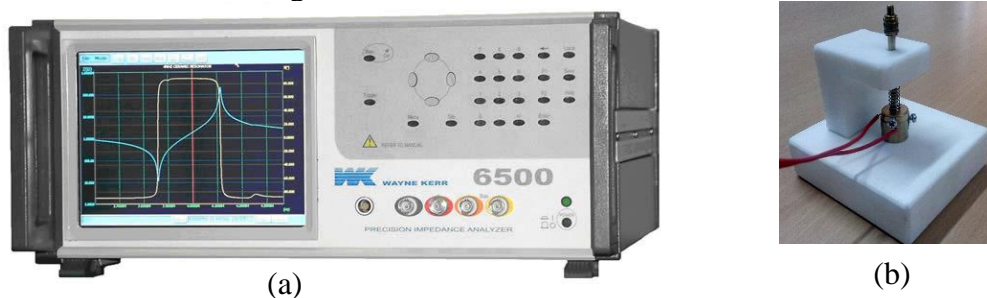
Fig 2.23 Instrumentation for dielectric studies: (a) Impedance analyser (b) Sample holder
