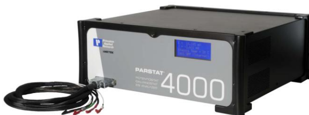
Fig 2.4 Electrochemical workstation (PARSTAT 4000) employed for PZT thin film deposition
