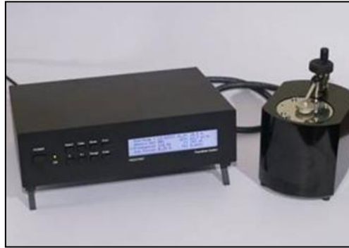
Fig 2.26 Piezometer used for measuring piezo properties
