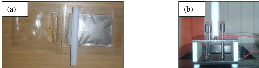
Fig 2.8 (a) Silver epoxy paste for electroding, (b) In-house designed Stainless steel-Teflon jig for poling
