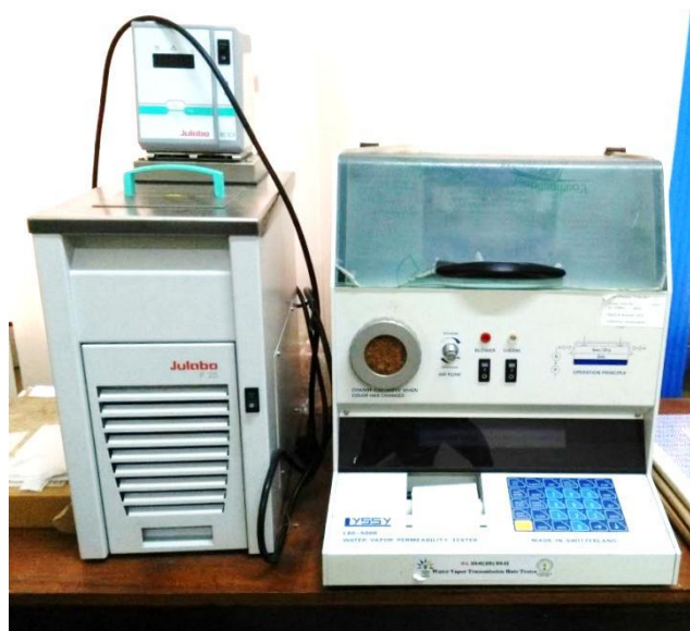
Plate 27 Lyssy L80-5000- Water vapour permeability tester (PBI Dansensor A/S, Ringsted, Denmark)
