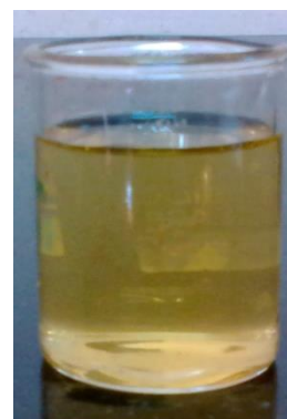
Plate 4 Liquid smoke produced from coconut fibre powder
