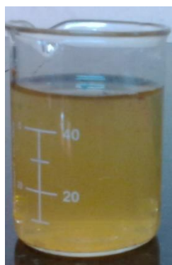
Plate 3 Liquid smoke produced from coconut fibre
