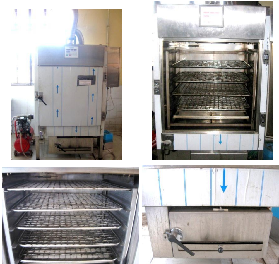
Plate 7 Multi-functional Smoke kiln
