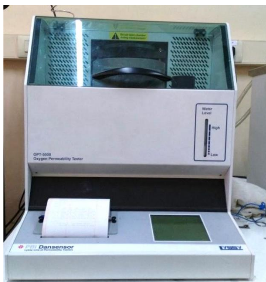
Plate 26 Lyssy OPT-5000-Oxygen permeability tester (PBI Dansensor A/S, Ringsted, Denmark)
