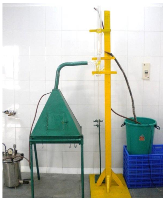
Plate 1 Indigenous liquid smoke production unit
