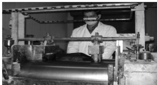
Fig.14 .Two roll mill for rubber mixing
