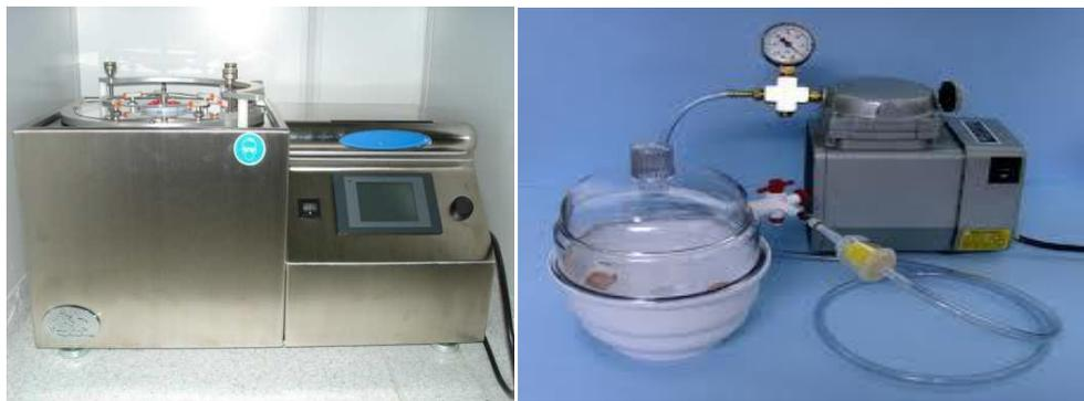
Fig 18: Programmable spin coater, Fig.19. Vacuum pump with desiccator
