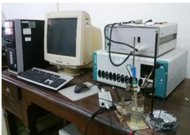
Fig. 22. EIS measurement setup Autolab PGSTAT30
