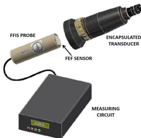
Fig.13. Schematic of the fringing electric field impedance probe with measuring circuit with a typical encapsulated transducer.
