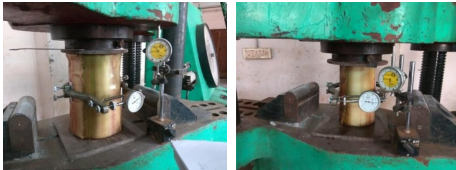
(a) Specimen, extensometers and load dial of the UTM
