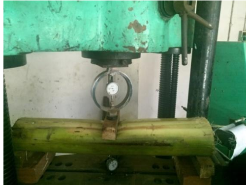
Fig. 2.2: Flexure test set-up of a banana specimen in the UTM, the proving ring, its dial and the dial gauge to measure deflection are also seen
