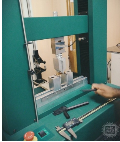
Figure 2.5 Universal testing machine under flexural tests
