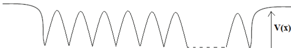
Fig 2.3 Periodic potential V(x) due to atomic core in a crystalline solid
