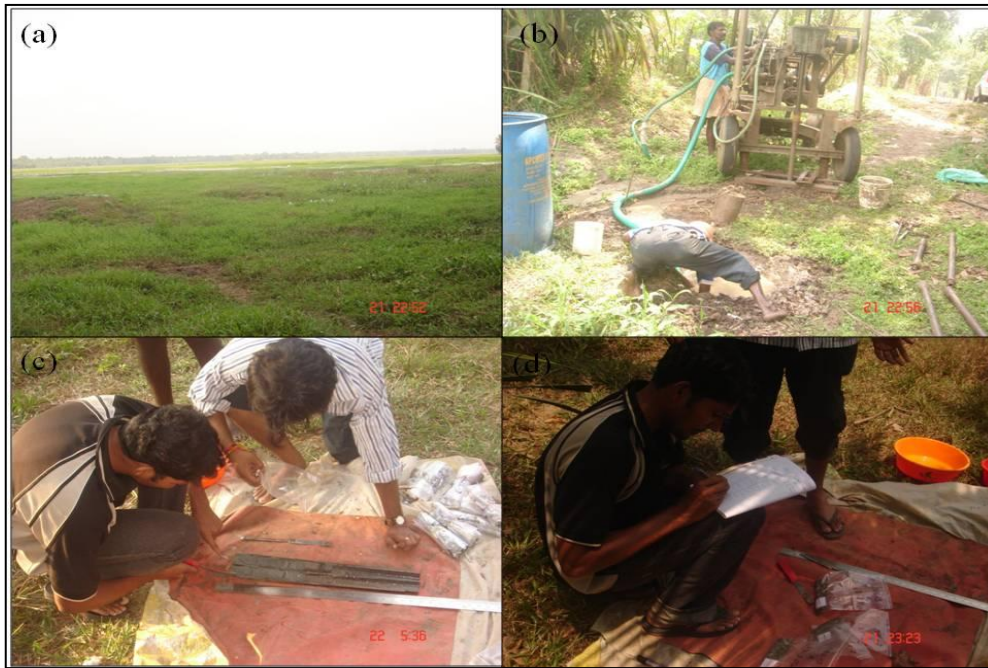
Fig. 3.3 Field photographs of core sample collection from the Kayamkulam coastal plain (northern boundary of the study area) showing (a) site area east of Kayamkulam Lagoon, (b) Rotary drilling in operation, (c) undisturbed sediment core and (d) lithological observation as well as packing of the samples
