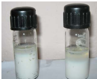
Fig. 3.17. Dispersions of clay made by sonication (left) and ball milling (right) after 5 weeks of preparation
