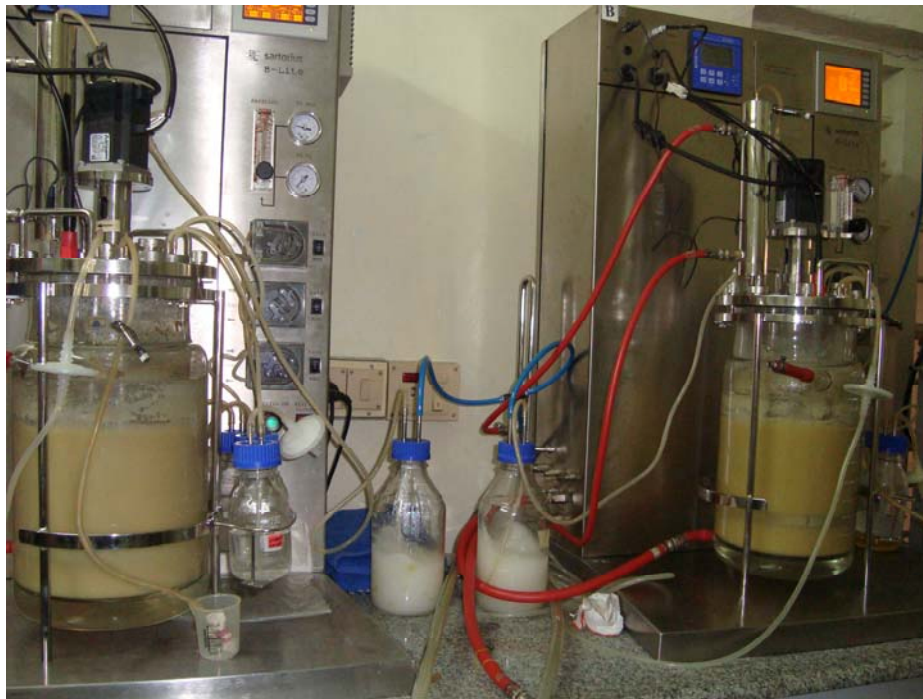
Fig.10 Biomass generation of Candida MCCF 101 in 5L bench top laboratory scale fermentor
