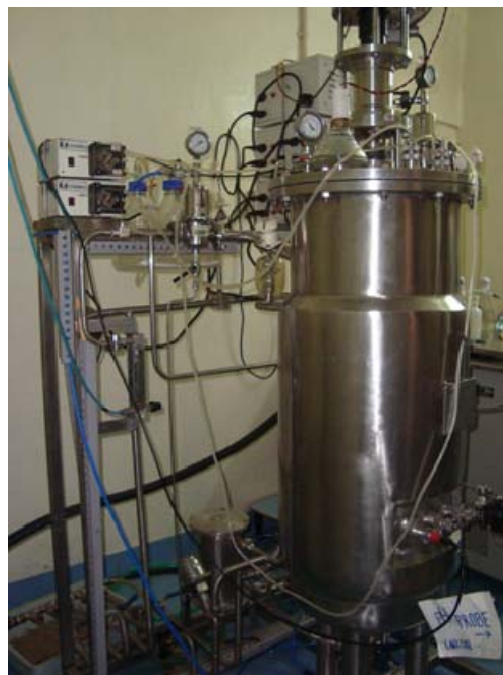
Fig.2 Pilot scale biomass generation in a 100L in situ sterilizable fermenter containing 75L using malt extract broth
