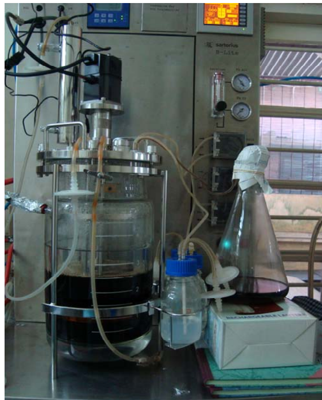
Fig.2 5L lab scale bench top fermentor containing molasses medium
