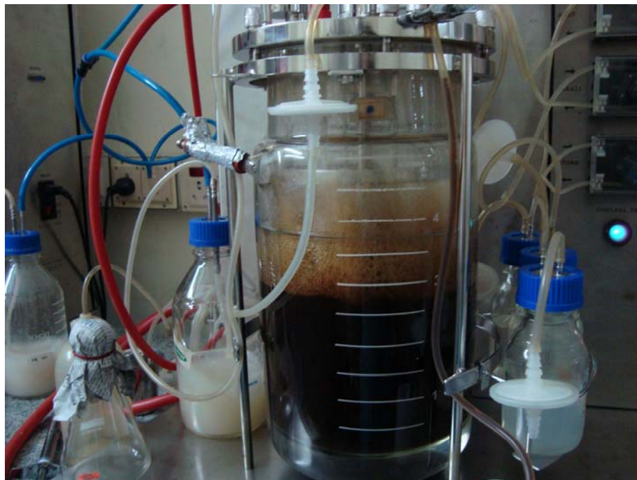
Fig.12 Biomass generation in laboratory scale fermentor using molasses based medium
