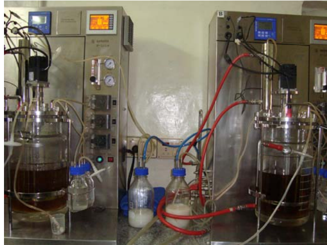
Fig. 1 5L lab scale bench top fermentor containing 3L mineral based medium for Biomass production of Candida MCCF 101
