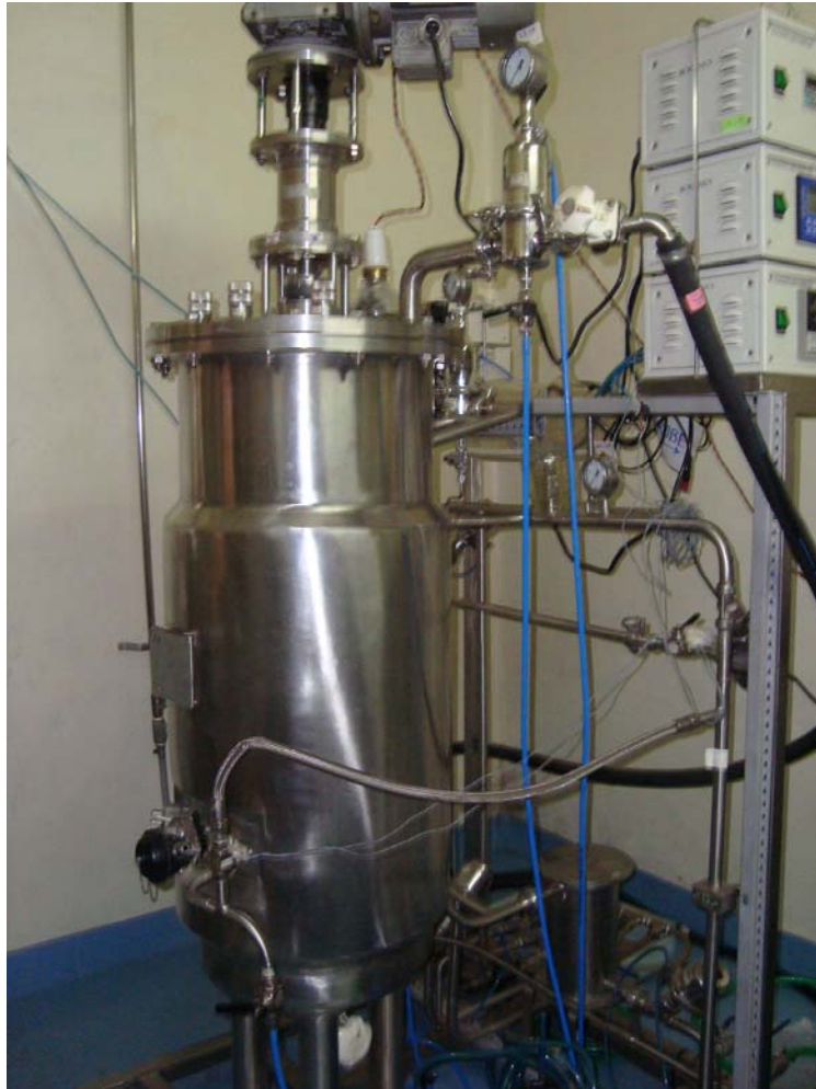
Fig. 3 Pilot scale 100L fermentor for scale up production of Candida MCCF 101
