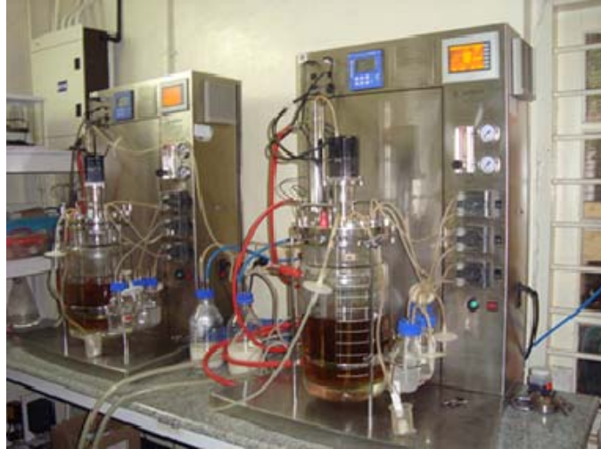
Fig.1 Biomass production in a 5L fermenter containing 3L malt extract broth
