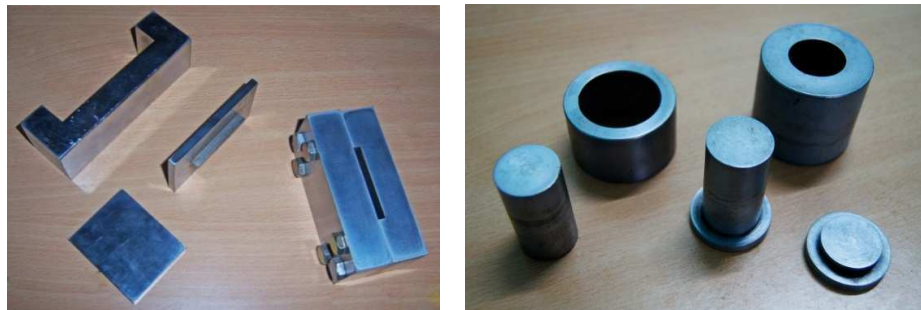
Figure 1.15 Rectangular and cylindrical dies designed for pelletizing samples
