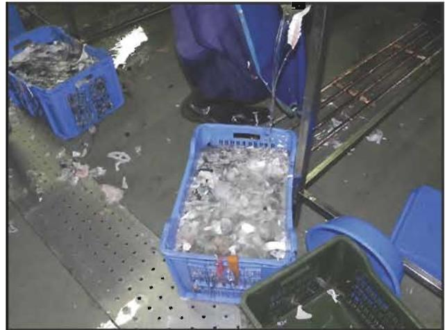
**3.4(b): Liquid and solid wastes being separated**
