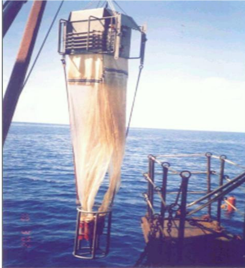
Plate 2.4. Multiple Plankton Net (MPN)
