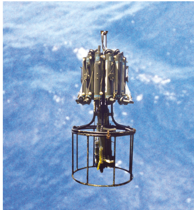
Plate 2.2. CTD rosette with Niskin bottles
