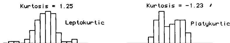
Figure 4.13: Two distributions having same variance and skew, but different kurtosis a) Leptokurtic distribution b) Platykurtic distribution
