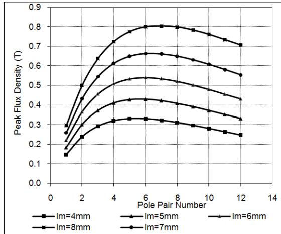
**Fig. 7:** Variation of peak  $B_{r1}$  with change in length of magnet and pole pairs (Analytical Results)
