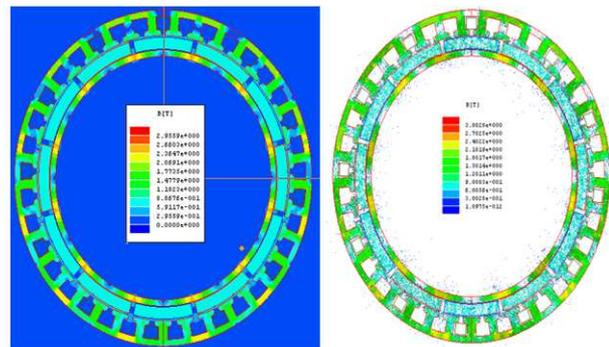
**Fig.3:** Flux Distribution of the optimized 37 slot, 12 pole PMLDC machine (FE Results)
