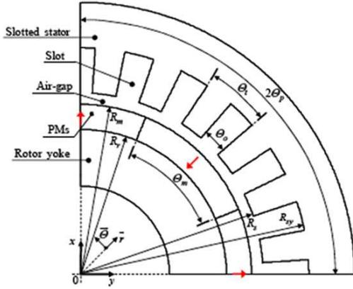
**Fig.1:** Cross section of a slotted PMBLDC Motor
