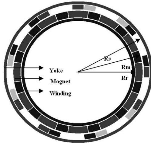
**Fig.6:** Zero Cogging PMBLDC Motor with Halbach array
