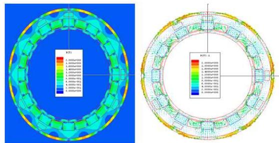
**Fig. 9:** Flux Distribution of the machine (FE Results)
