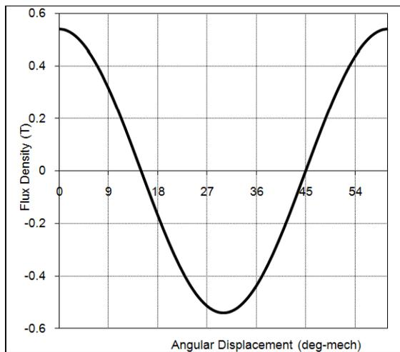
**Fig. 8:** Variation of mean air gap flux density under one polepitch (Analytical Results)
