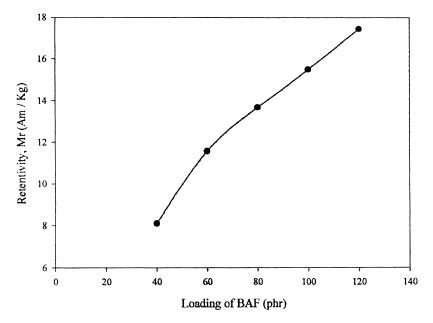
FIGURE 5 Retentivity versus loading of fillers.
