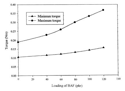
FIGURE 2 Minimum torque and maximum torque versus loading of fillers.
