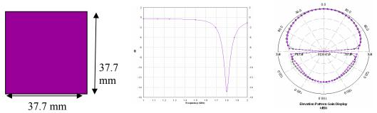
Figure.4 37.7x37.7mm square patch, R.L curve and radiation pattern
