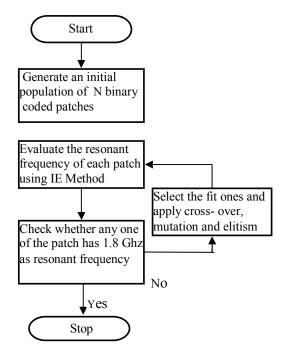
Figure.1 A simple flowchart for microstrip antenna design using GA
