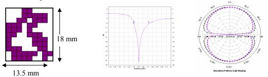
Figure.7 The final Genetic patch with optimized GP, R.L curve and Radiation Pattern
