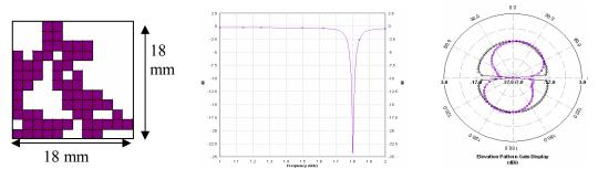
Figure.5 18x18 mm patch, R.L curve and Radiation pattern
