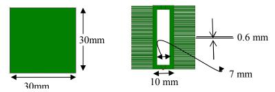
Figure.6 Ground plane 30mm x30mm before and after optimization
