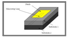
Figure.2. An electromagnetically coupled MSA
