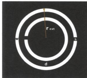
Fig.4. Two Ring SRR with variables External radius ( $R_{ext}$ ), Width of ring( $w$ ), Gap between rings( $d$ ), Height of substrate ( $h$ ), Relative permittivity of substrate ( $\epsilon_r$ ), Width of slit in ring( $s$ ). Reference dimension chosen is  $R_{ext}$ =6mm;  $w$ =0.3mm;  $d$ =0.3mm;  $s$ =0.3mm;  $h$ =1.6mm; and  $\epsilon_r$  =4.4
