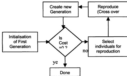
Fig.1. Genetic Algorithm flowchart
