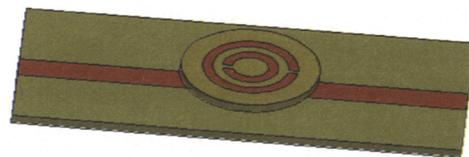
Fig.2. SRR coupled to Microstrip transmission line
